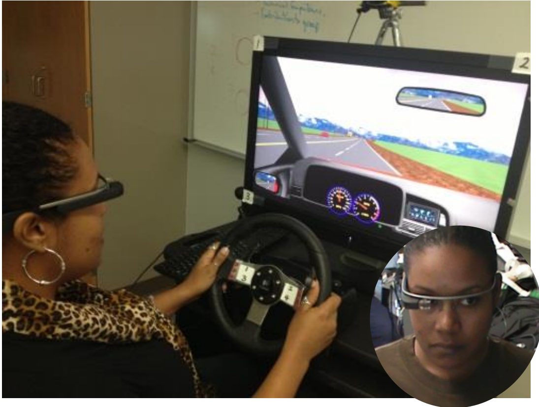
Figure 9. Experimental setup in the Glass texting condition. In conditions involving smartphone interaction, the device was placed on the table near the mouse. The picture in the right-hand corner is a still shot from the video recordings collected and used for coding the eye movement data.
