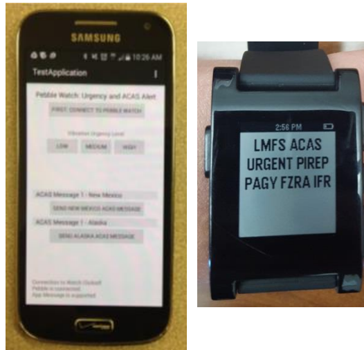
Figure 18. Pebble smartwatch display. (Left) The smartphone software controller. (Right) An example text of the ACAS alert summary.
