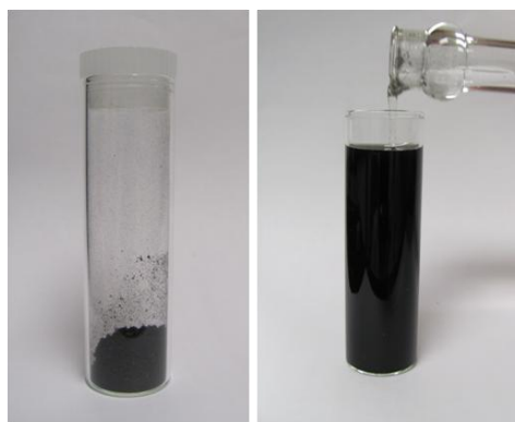
Figure 4.11. Redispersion of freeze-dried Py-SASS/graphene powder in water at original dispersion concentration.
