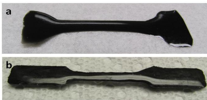
Figure 4.15. 0.5 wt % graphene/epoxy composites prepared by a) Doctor-blading and b) casting in a Teflon mold.
