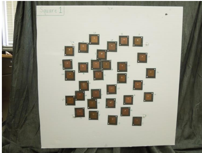
Figure 140. Thirty two element square patch random antenna array.
