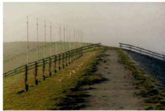
Figure 5. High frequency (HF) codar random array application. [106]
