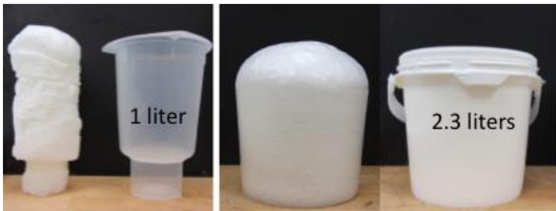
Figure 34: Comparison of the volume and dimensional stability of foams from the original process (left), to those from the modified process (right).
