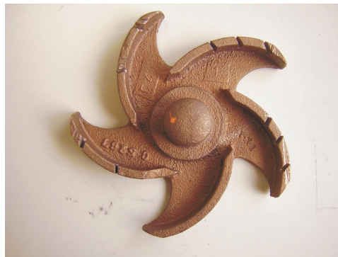
Fig. 27. Photograph of the staged impeller cracks.
