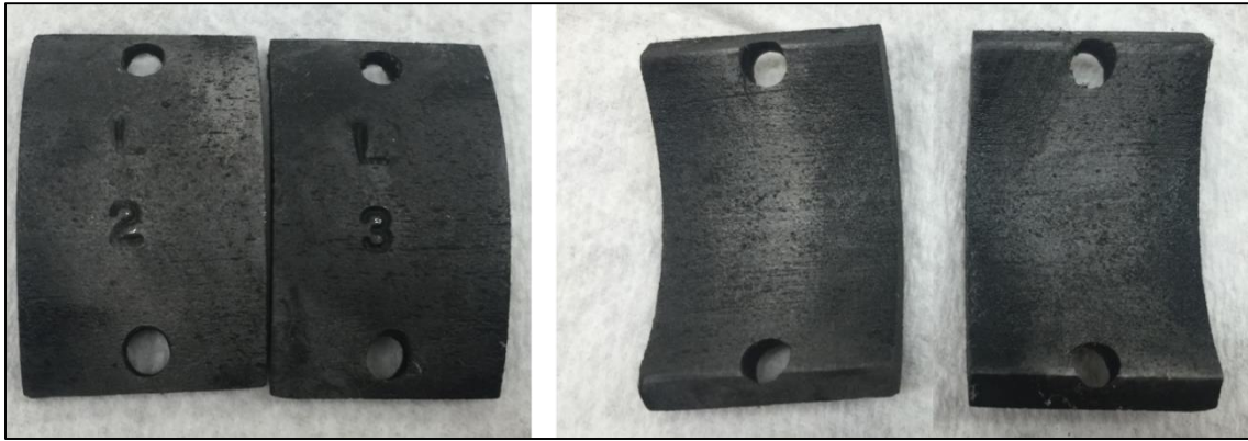
Fig. 8 – Results of L-80 test with 20 wt% GLDA (pH = 4). Coupon after corrosion outer side surface (left) and inner side surface (right). Test was conducted for 4 hours at >1000 psi at 300°F.
