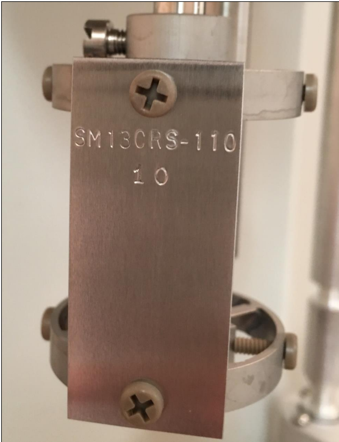
Fig. 4 – Parr reactor (coupon holder).
