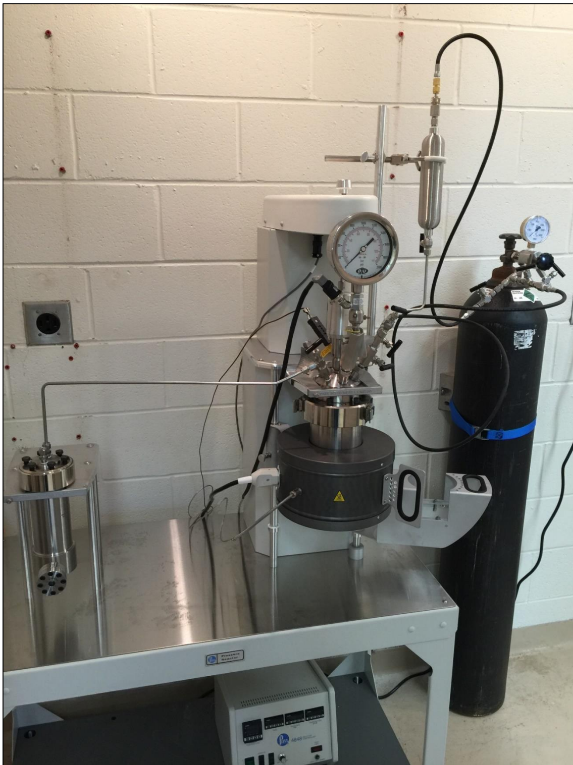
Fig. 3 – Parr instrument reactor system assembled.
