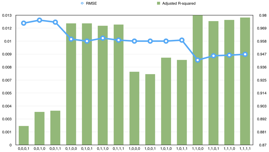
Figure 3.4: Adjusted R-squared and RMSE for the set of variables \{l1 \text{ data MPKI}, l2 \text{ data MPKI}, LQFullEvents, tlb \text{ MPKI}\} with 1 indicating the presence and 0 indicating the absence of the variable
