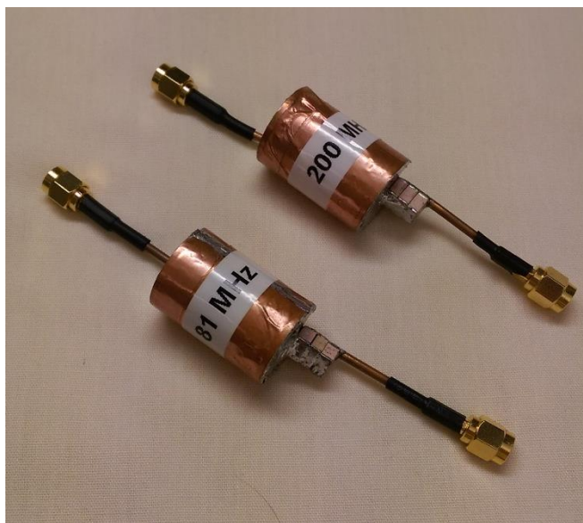
Figure 3.7 Baluns Tuned to the ^1\text{H} and ^{31}\text{P} Frequencies for 4.7T. These are 200.079 MHz and 81.005 MHz, respectively.
