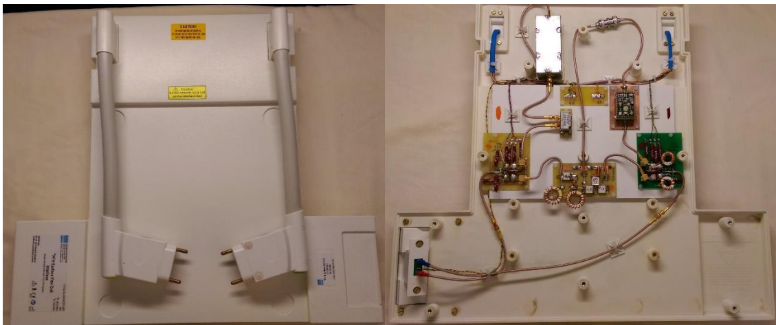
Figure 4.5 Interface Box for 3T Coil. This interface box produced by RAPID MR International showing the outer casing ( left ) and the inner components ( right ). The box contains several built-in receive-line components including TR switches for each channel, pre-amplifiers for each channel, and a frequency splitter.
