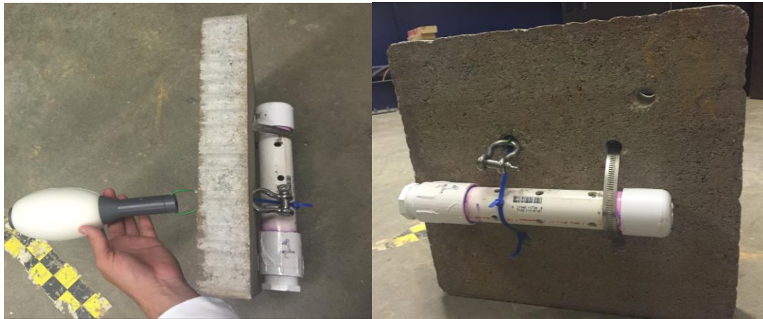
Figure 3. (a) Concrete base of the instrument pod (view from above), and (b) TCM mooring system.
