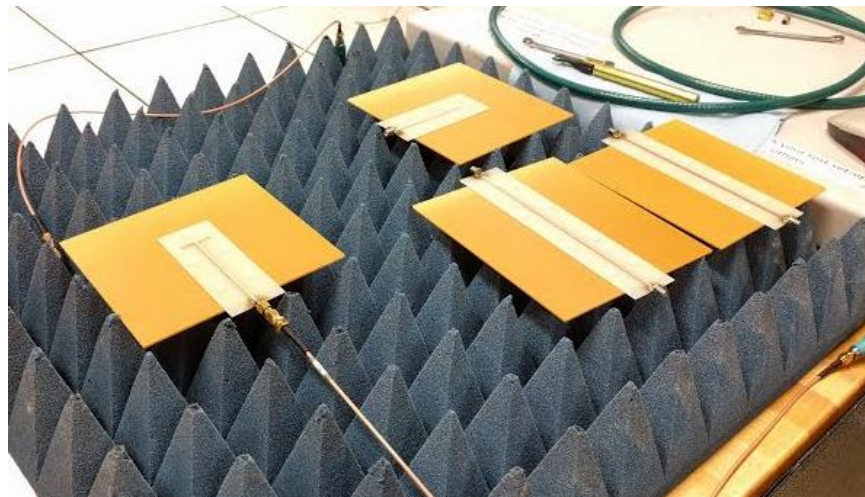
Figure 18. LMA (left), Reflect standard (top middle), Line Standard (bottom middle), Thru Standard (right)
