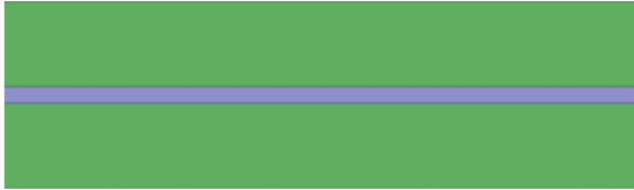
Figure 11. Parallel Strip TL, the dark grey is on the bottom of the substrate (not shown) and the purple is on top of the substrate
