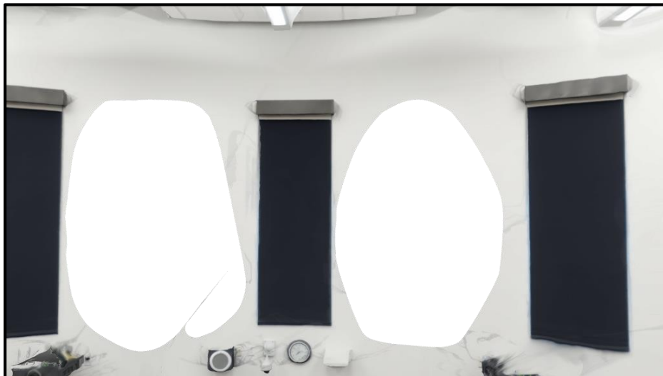
Figure 5.5: Holes appear on bright texture-less walls in section 7
