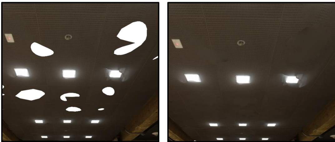
Figure 3.34: Fixing the holes in the mesh model by the same texture
