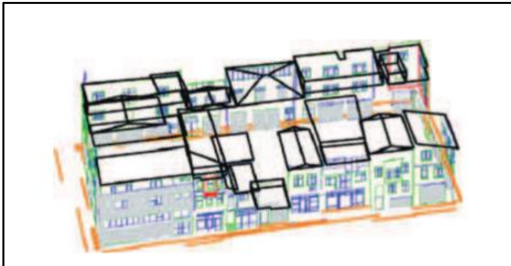
Figure 2.7: Using aerial photogrammetry to produce roofs and terrestrial laser scanners to produce the walls in a neighborhood in Istanbul, Turkey (Kesten et al. 2009)
