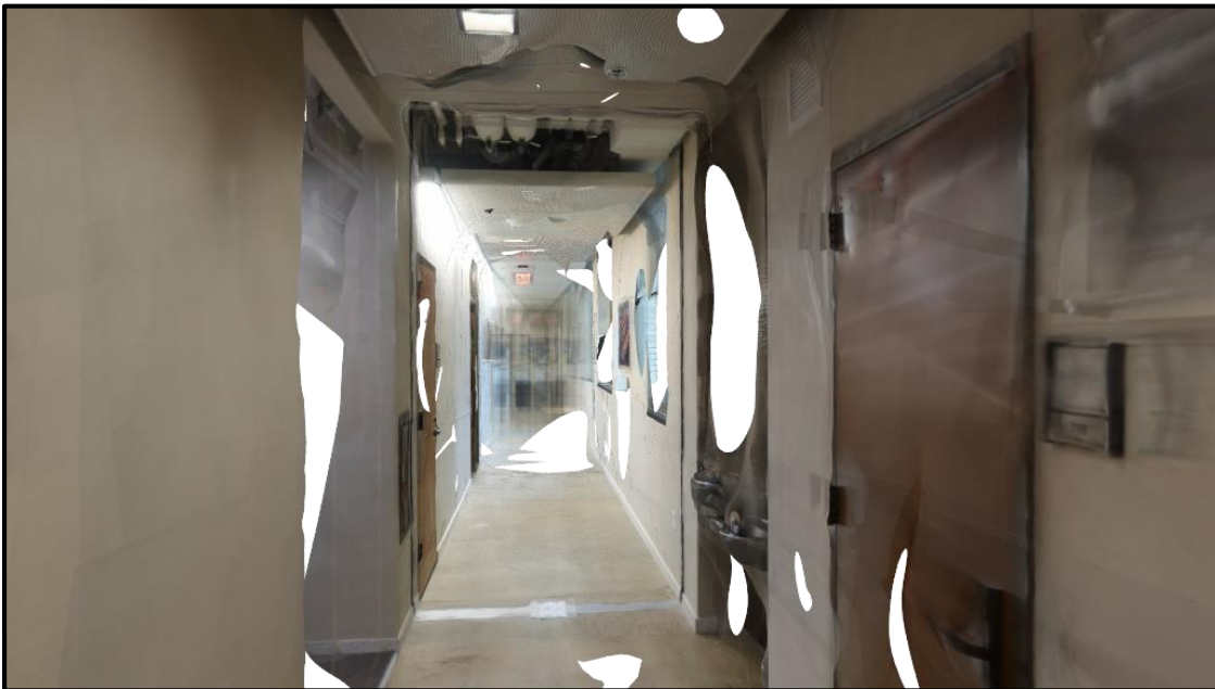
Figure B.6: Section 8 mesh model extracted from Autodesk Recap
