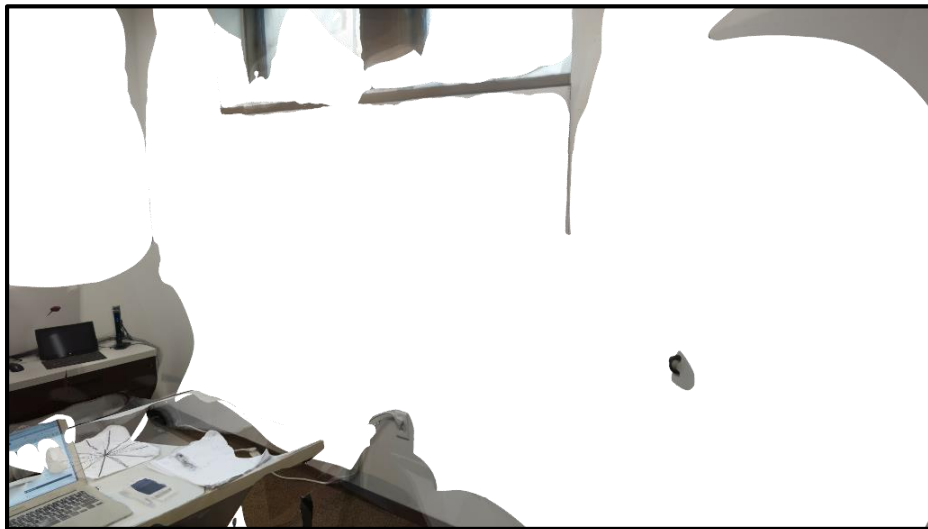
Figure 5.9: Incomplete surfaces in section 14
