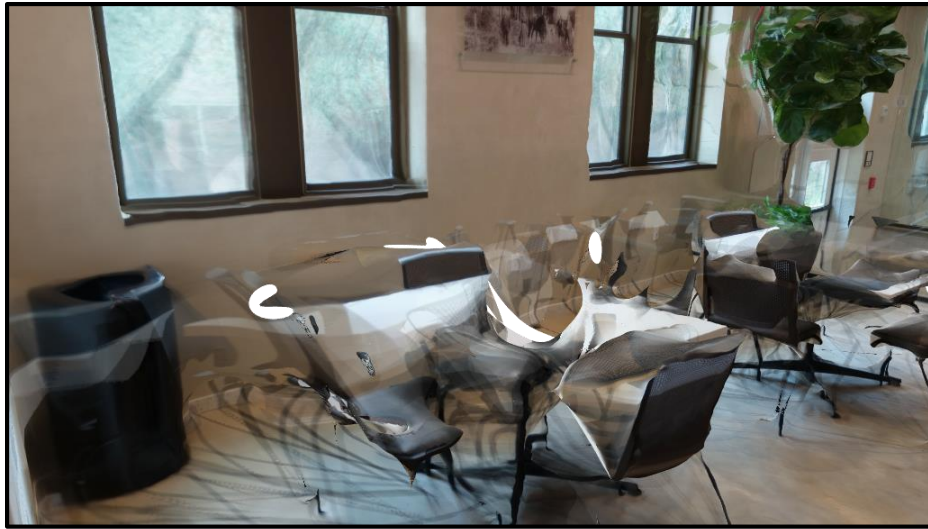
Figure 5.13: Deformation of meshes in section 2 due to presence of furniture
