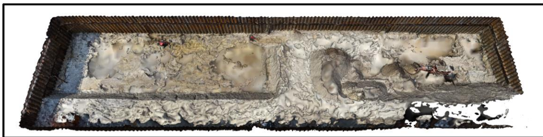
Figure 2.4: 3D model of excavated jobsite using photos (Borrmann et al. 2013)
