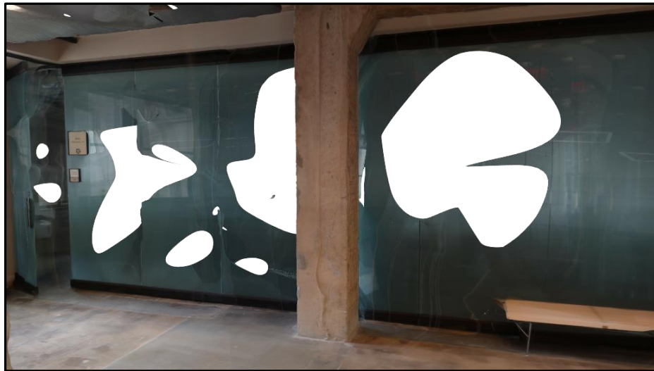
Figure 5.6: Holes appear on reflective glass surfaces in section 1
