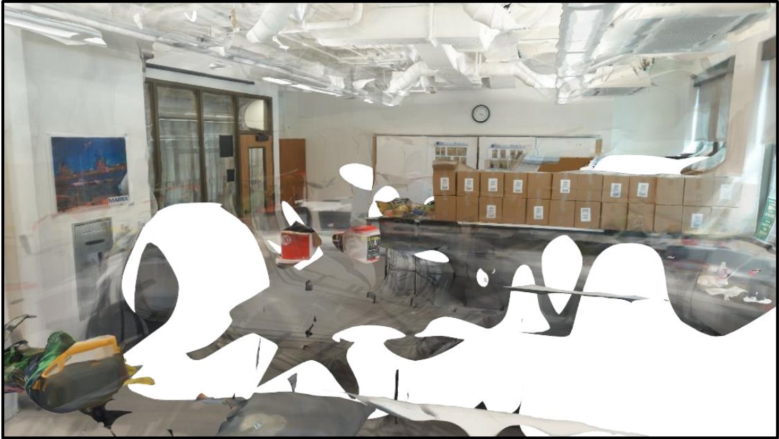
Figure B.9: Section 11 mesh model extracted from Autodesk Recap
