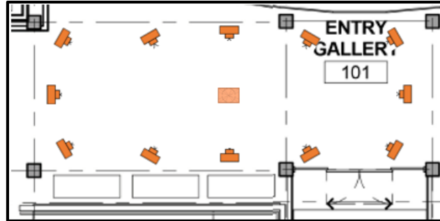
Figure A.1: Section 3 camera placement diagram (B. R. W. Architects 2013)
