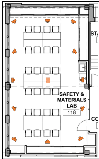
Figure A.8: Section 11 camera placement diagram (B. R. W. Architects 2013)
