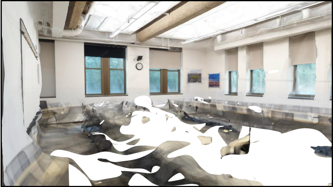
Figure B.13: Section 15 mesh model extracted from Autodesk Recap
