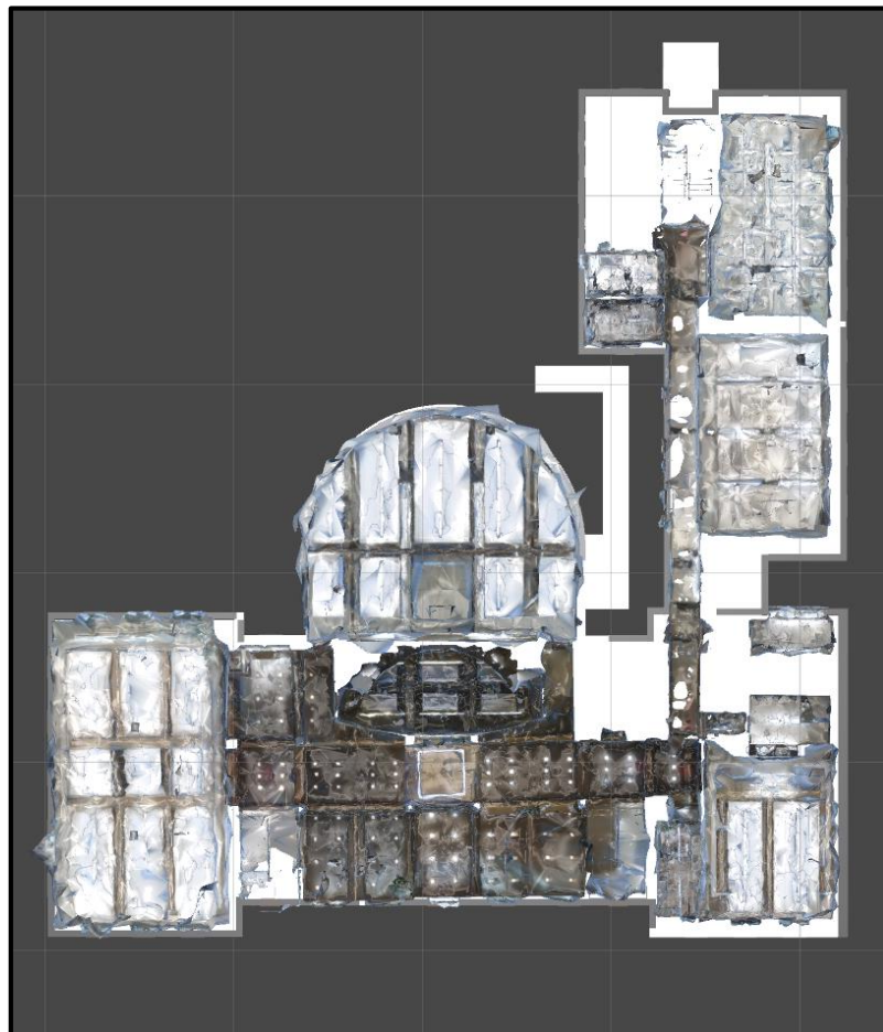
Figure 5.19: BIM model overlaid on the stitched model
