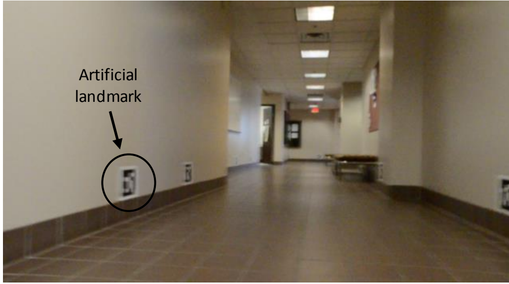
Figure 4.4: Sample image frame where visible artificial landmarks are used to compute the ground-truth camera position.
