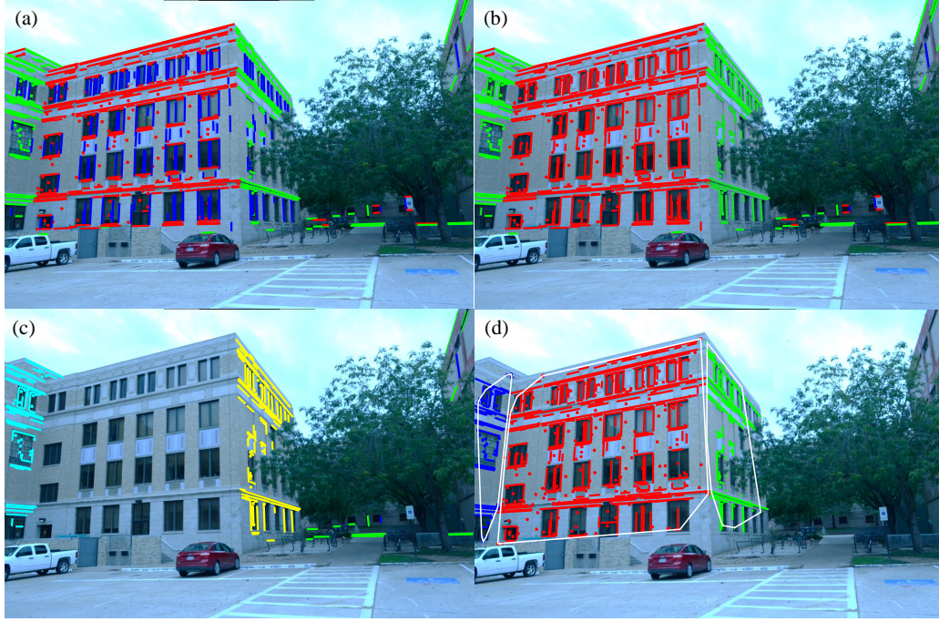
Figure 3.4: Extracting PBFs. (a) Feature points associated to vanishing direction of neighboring (color-coded) horizontal line segments. (b) Vertical line segments associated to vanishing direction of neighboring (color-coded) horizontal line segments. (c) Homography clustering applied to feature points with same vanishing direction. (d) Convex hull for each homography cluster.
