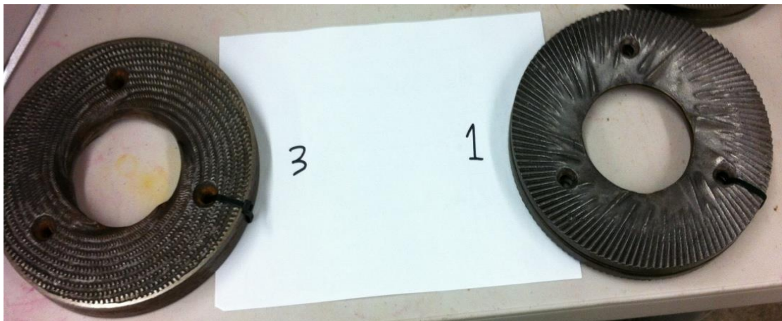
Figure 6. Plate 3 (left) is a less aggressive plate while plate 1 (right) is a more aggressive plate.
