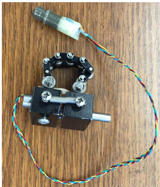
Figure 15: Radial LVDT and chain
