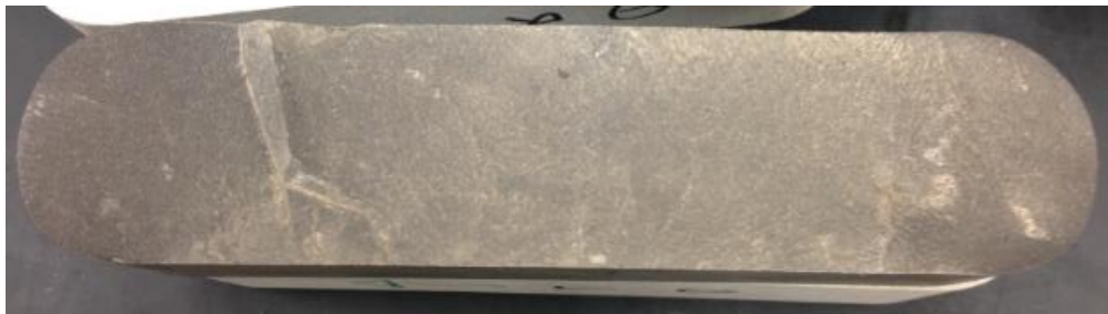
Figure 43: Fracture surface of facies B1 perpendicular conductivity sample (Tenorio, 2016)
