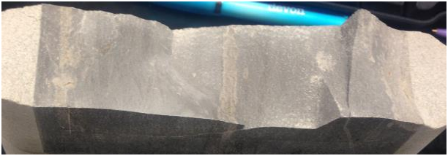
Figure 58: Fracture surface of facies C parallel conductivity sample (Tenorio, 2016)
