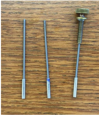
Figure 13: Ferromagnetic cores used in triaxial testing
