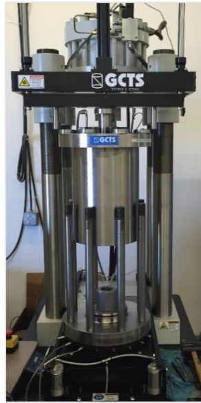
Figure 8: The triaxial cell
