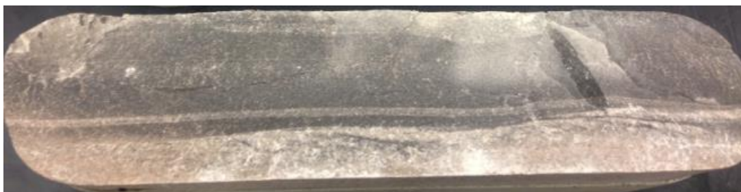
Figure 81: Fracture surface of facies A parallel conductivity sample (Tenorio, 2016)
