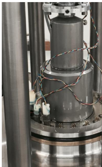
Figure 9: LVDTs connections at base of triaxial cell
