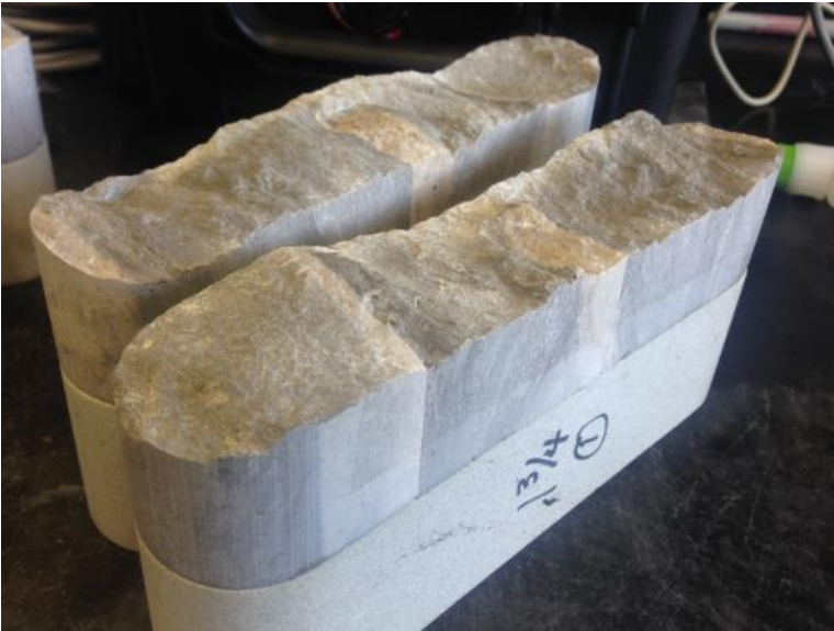
Figure 72: Fracture surface of facies E parallel conductivity sample (Tenorio, 2016)
