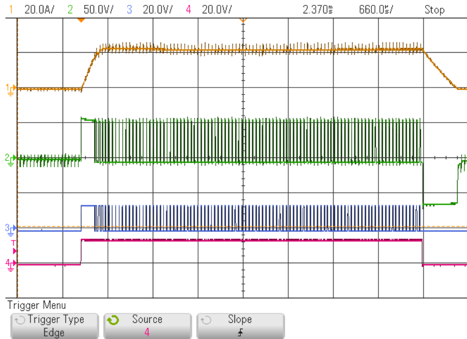
Fig. 5.11 Current, voltage and switching signals
