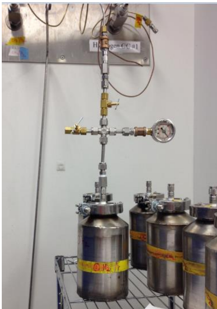
Figure 4.3 Stainless steel fermentors being filled with desired gas and headspace pressure.
