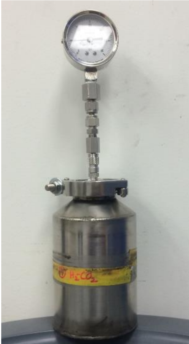
Figure 4.2 Stainless steel fermentor with a pressure guage.
