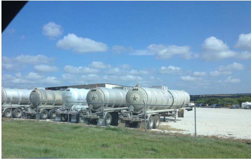
Figure 5: These truck trailers are used to transport water to the drill site for fracking. After fracking is complete, these trucks often carry “produced water” (also referred to as “saltwater”) to injection wells or treatment sites. On average, seven to ten barrels of water are brought to the surface for every barrel of oil extracted (Guerra, Dahm, and Dundorf 2011). Each of these trailers can transport approximately 190 barrels of liquid per trip. (Photo courtesy of the author.)
