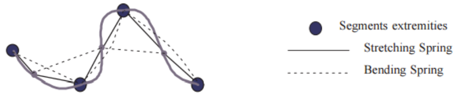
Figure 2.5: Spring distribution over a spline in the work by Lenoir et al. [24]. The stretching and bending behavior are achieved through the stretching springs and bending springs. Twisting are not considered.
