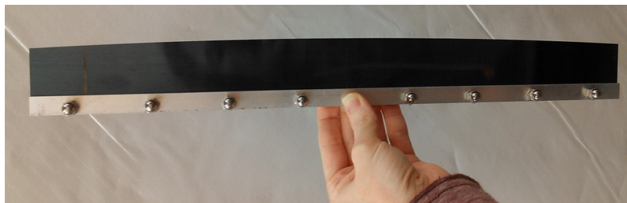
Figure 4.17: A pusher bar for holding the wires in the curve along the top and bottom of the BTC during winding.
