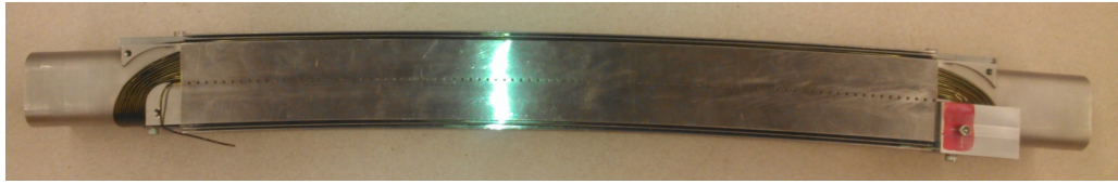
Figure 4.15: Top view of the updated winding mandrel and one of the temporary aluminum winding guides on the endcap.
