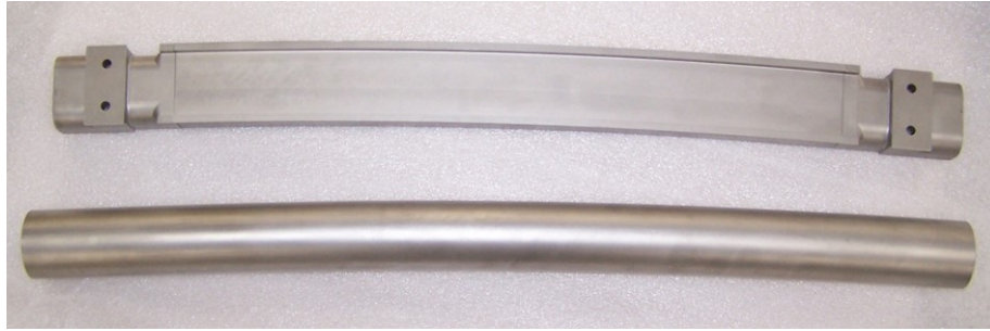
Figure 4.11: Initial curved mandrel and beam pipe
