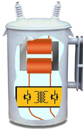
Figure 7. Concept of Smart Distribution Transformer Scheme Including Power Electronics Module for Smart Grid.
