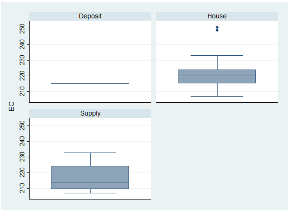
Figure 22 Box and whisker plots of electrical conductivity (EC) in water samples. N=26
