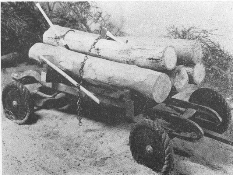
Fig. 8. Two cross bunks fastened to automobile chassis make an easy pulling light log wagon.
