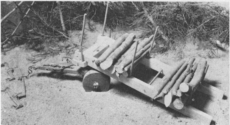
Fig. 9. One way to save trucks and farm wagons is to bunch pulpwood or firewood along woods roads with a wood rack; front end can be carried on a bumper with bolster.
