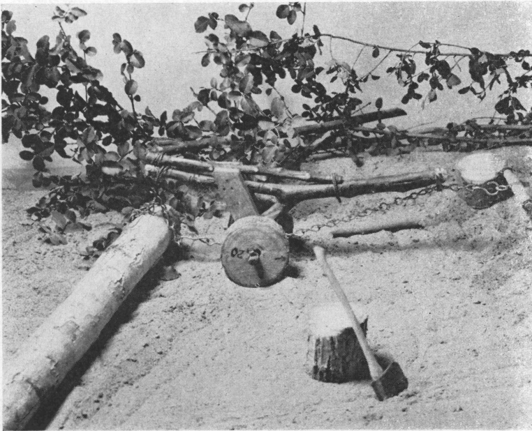
FIG. 17. This is a lazy bumper, an experimental device which raises log end only when pulled.
