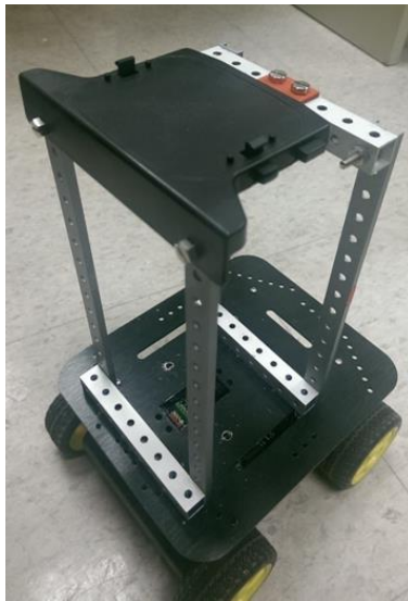
Figure 2-3 The structure to carry the Kinect sensor
