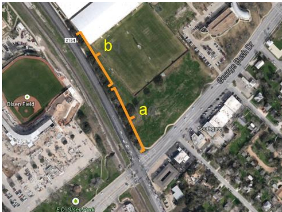
(a) is the comprehensive waiting area (b) is a segment before pre-signals where vehicles wait before entering CWAs Figure 12 The Studied Intersection with a CWA on the southbound Approach.
