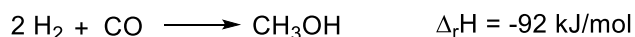
Figure 1.2 Fischer-Tropsch reaction for synthesis of heavier alkanes from syngas and conversion of methane to methanol via syngas.
