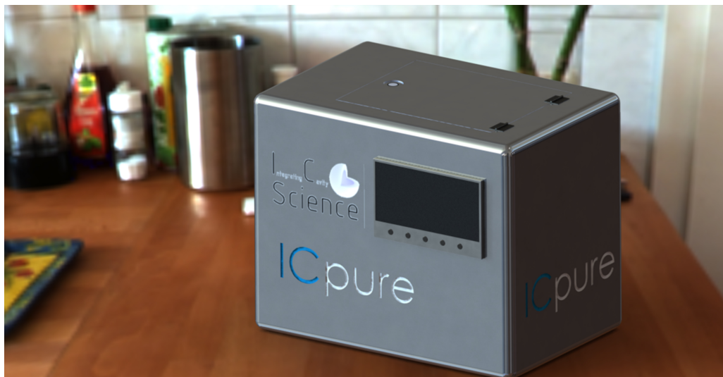
Figure 7.1: Conceptual rendering of an integrating cavity based water analysis system
