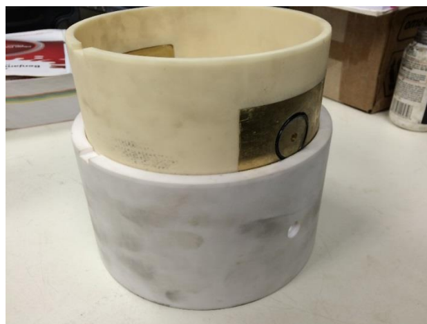
Figure 32. Insertion of inner alumina ring into outer with electrodes in place
