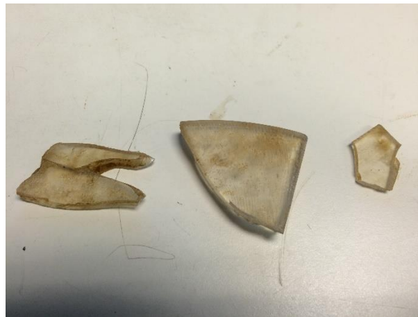
Figure 51. Plastic pieces discovered during disassembly of MPFM
