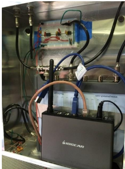
Figure 18. Inside of MPFM circuitry box with filter circuit, USB-to-ethernet converter/extender, and Picoscope signal generator/digital oscilloscope
