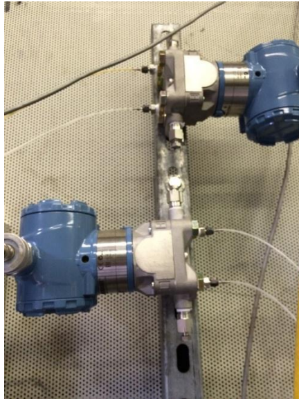
Figure 9. Rosemount pressure transducers used to measure slotted plate and venturi differential pressures
