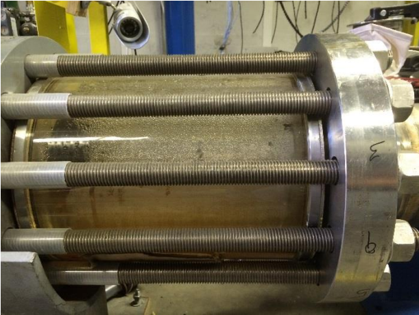
Figure 24. Acrylic visualization window for water line with CCTV camera visible
