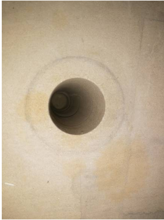
Figure 6.12: Wellbore after drilling
