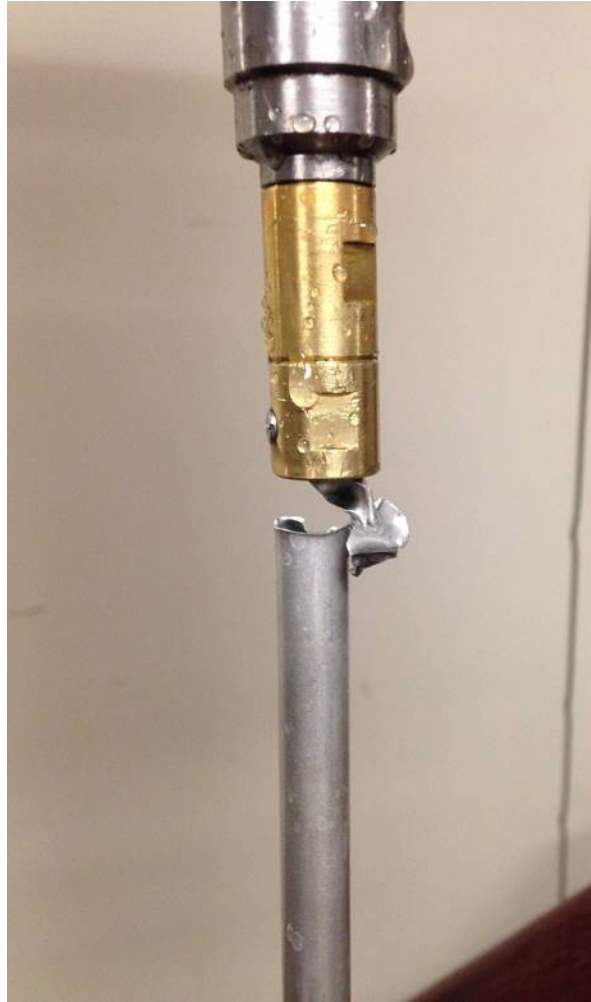
Figure 6.11: Drill pipe broken at the joint while drilling granite formation
