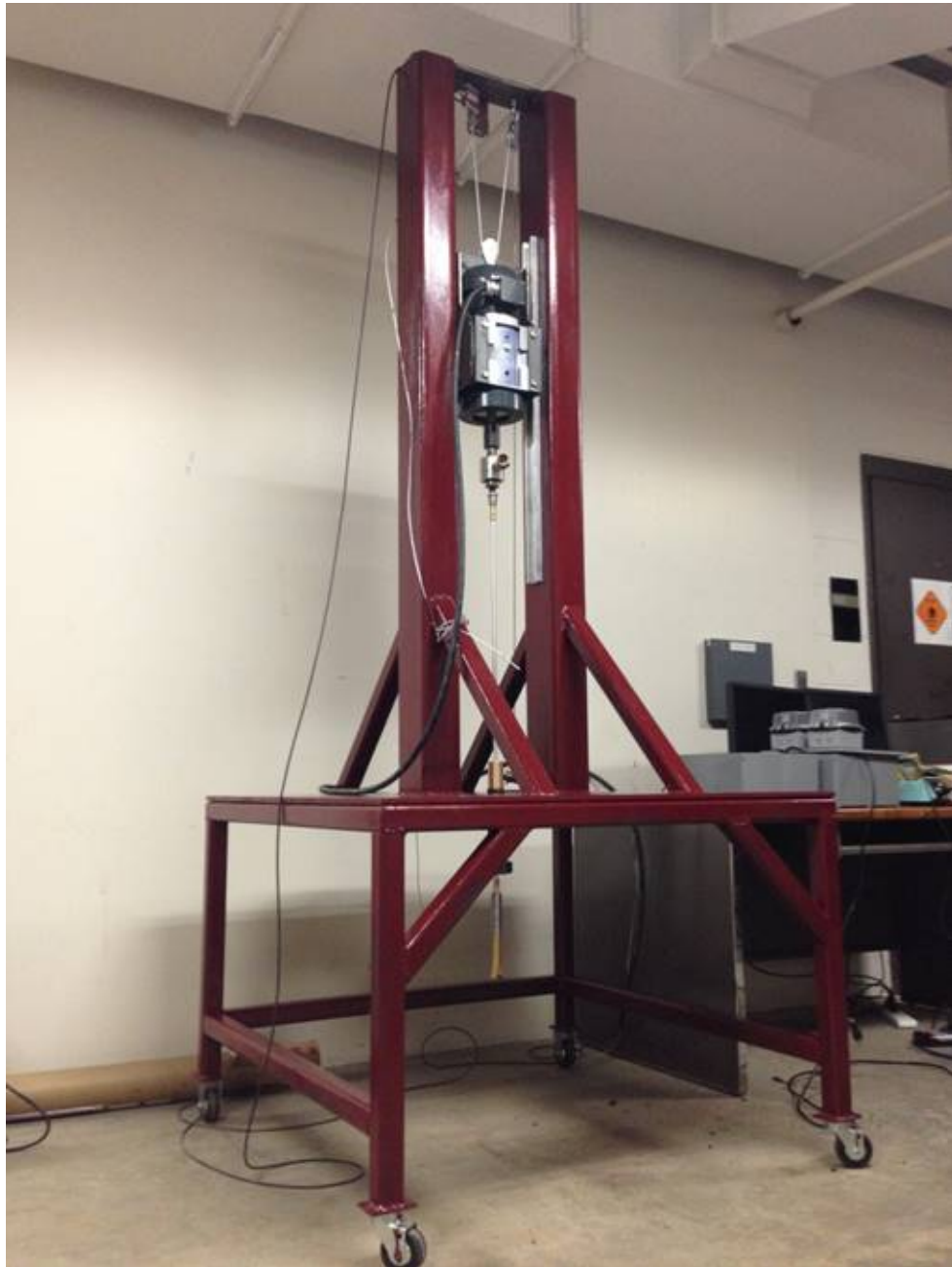
Figure 5.2: Miniature autonomous model drilling rig
