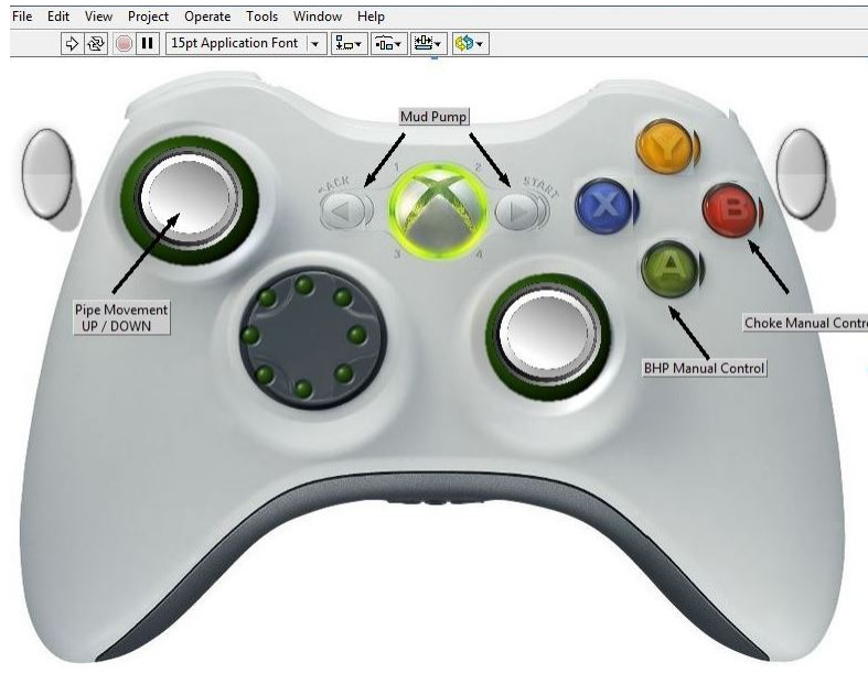
Figure 4.7: Drilling Simulator operated using joystick
