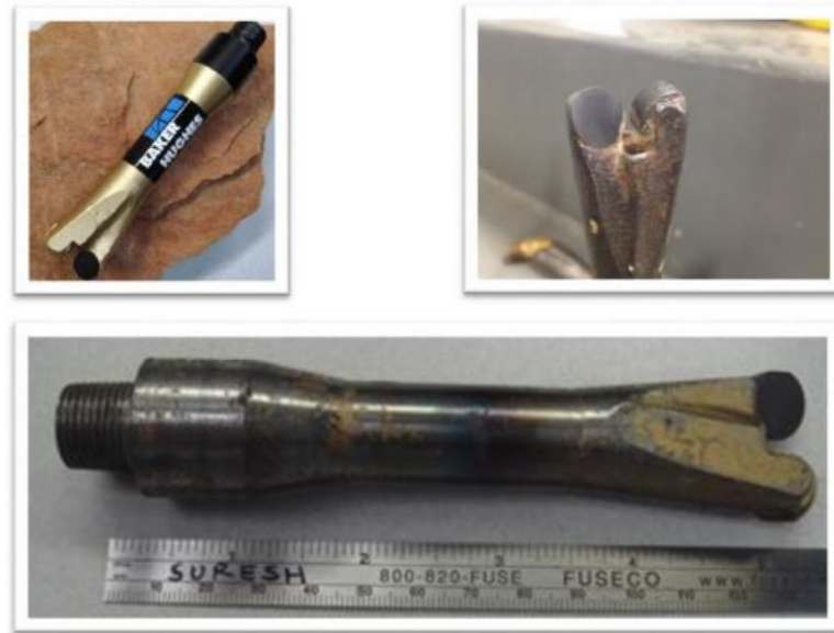
Figure 6.8: Drill bit used to drill the formation
