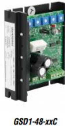
Figure 5.8: DC drives to control motors (Source:www.omega.com)
