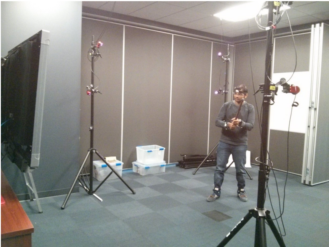
Figure 1 : Optitrack motion capture setup with Flex 13 cameras
