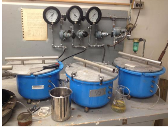
Figure 3.8. Pressure plate extraction vessels (-10,- 33, -100 kPa pressure vessels).
