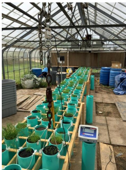
Figure 4.2. Greenhouse weighing apparatus. Consisted of a hanging load cell (1 g resolution) attached to a lockable lever load binder which allowed the researched to lift the column just enough to weigh it.
