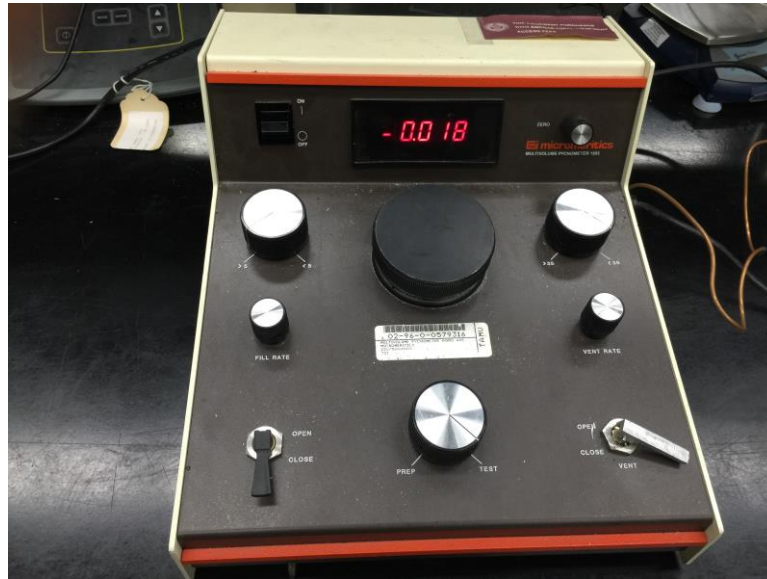
Figure 3.9. Micromeritics helium pycnometer used to calculate particle density.
