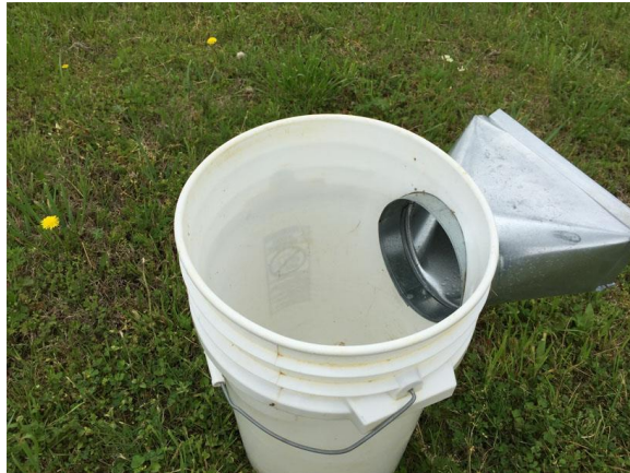
Figure 3.3. The runoff catchment device: 30 cm diameter by 50 cm tall bucket with embedded weir (before being sealed together and buried).
