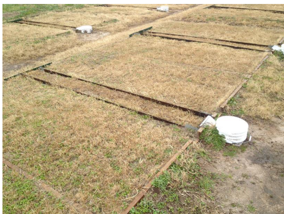
Figure 3.2. The center runoff/biomass collection plot, weir, and the buried buckets (which contain plastic bags to catch runoff).
