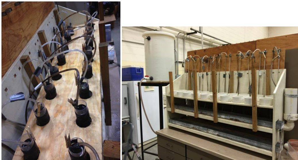
Figure 3.7. Constant head infiltrometer bench. Left: shown with sample columns being tested for K_{\text{sat}} . Right: front view of infiltrometer.
