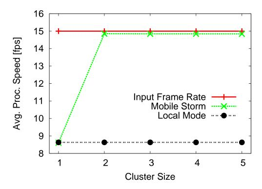
Figure 4.2: Processing speed of Mobile Storm and Local Mode for a video stream at  $1280 \times 720$  resolution
