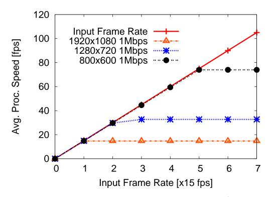
Figure 4.9: Processing speed change while increasing the input frame rate when cluster size=4
