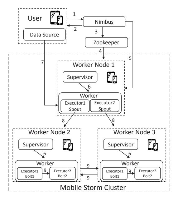
Figure 2.5: Steps for executing a job in a Mobile Storm Cluster
