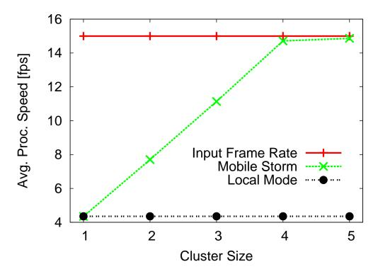
Figure 4.1: Processing speed of Mobile Storm and Local Mode for a video stream at  $1920 \times 1080$  resolution
