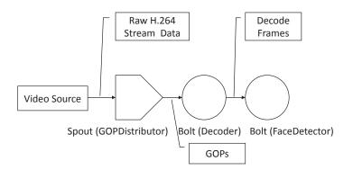
Figure 3.2: Mobile Storm Topology used in our evaluation
