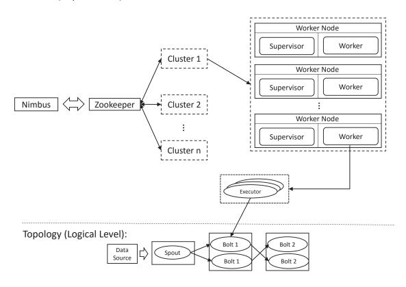
Figure 2.1: The logical and physical design levels for Mobile Storm
