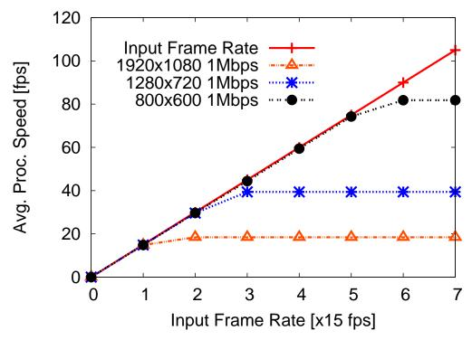
Figure 4.10: Processing speed change while increasing the input frame rate when cluster size=5
