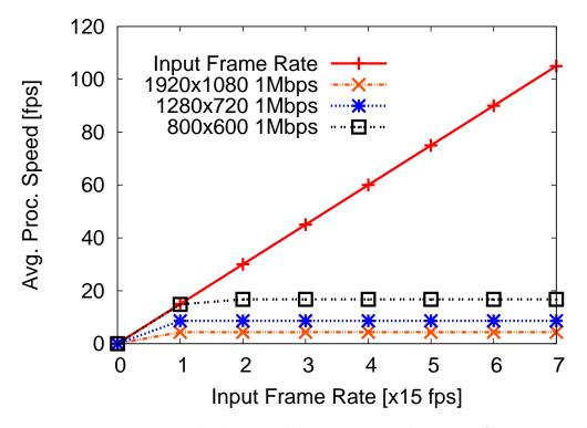
Figure 4.6: Processing speed change while increasing the input frame rate when cluster size=1
