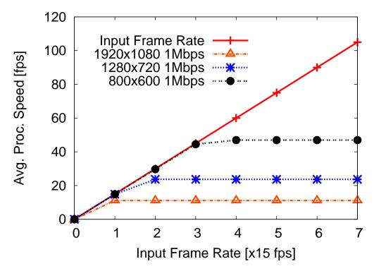
Figure 4.8: Processing speed change while increasing the input frame rate when cluster size=3
