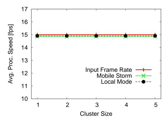
Figure 4.3: Processing speed of Mobile Storm and Local Mode for a video stream at  $800 \times 600$  resolution
