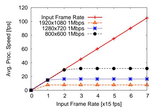
Figure 4.7: Processing speed change while increasing the input frame rate when cluster size=2
