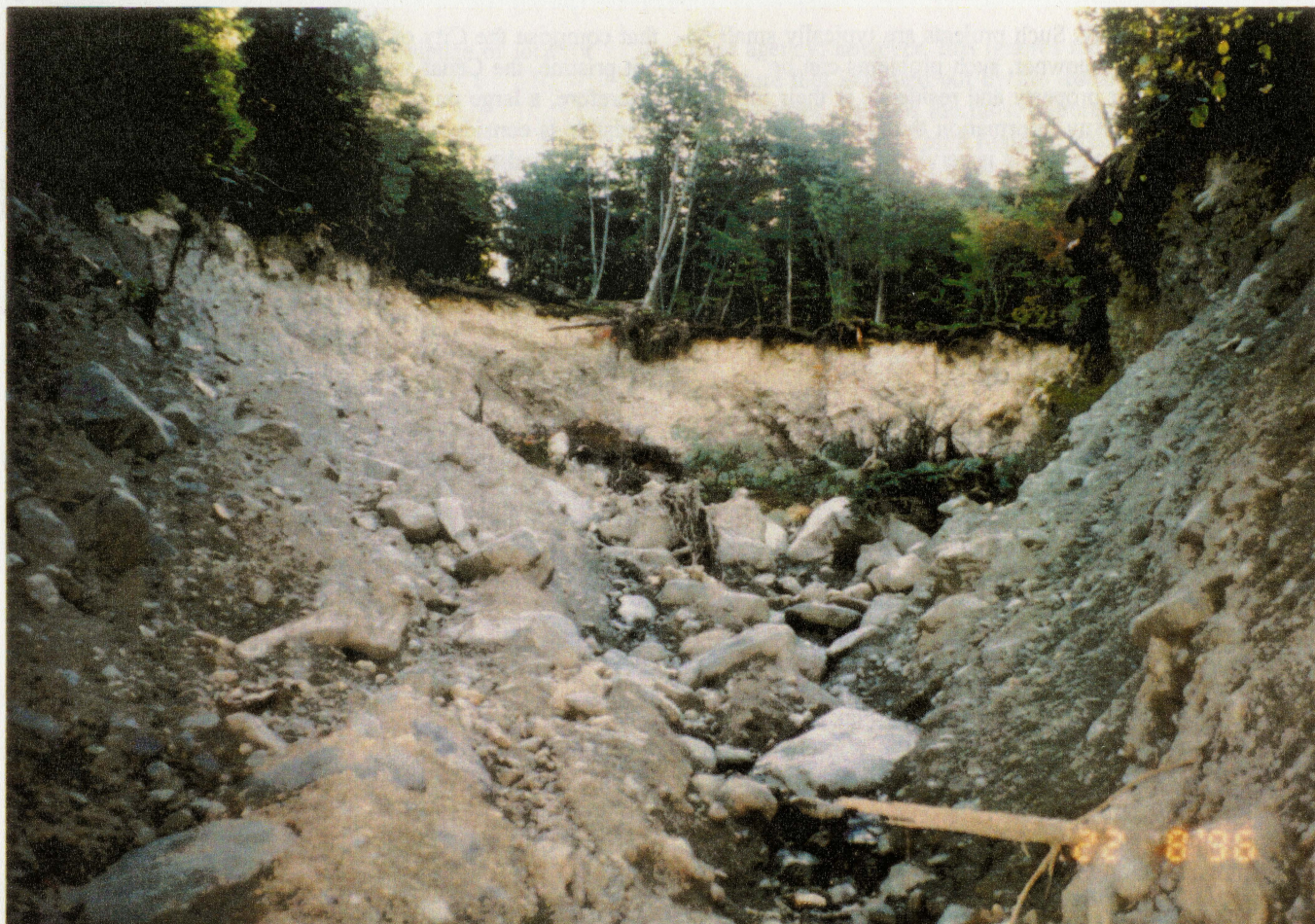
Figure 1. Longitudinal view of landslide in alpine till with smectite fine-grained particles. Headscarp in background is about 20 feet high.
