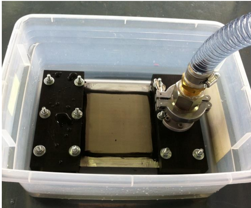
Figure 96. Membrane Cassette #3 water test experimental setup
