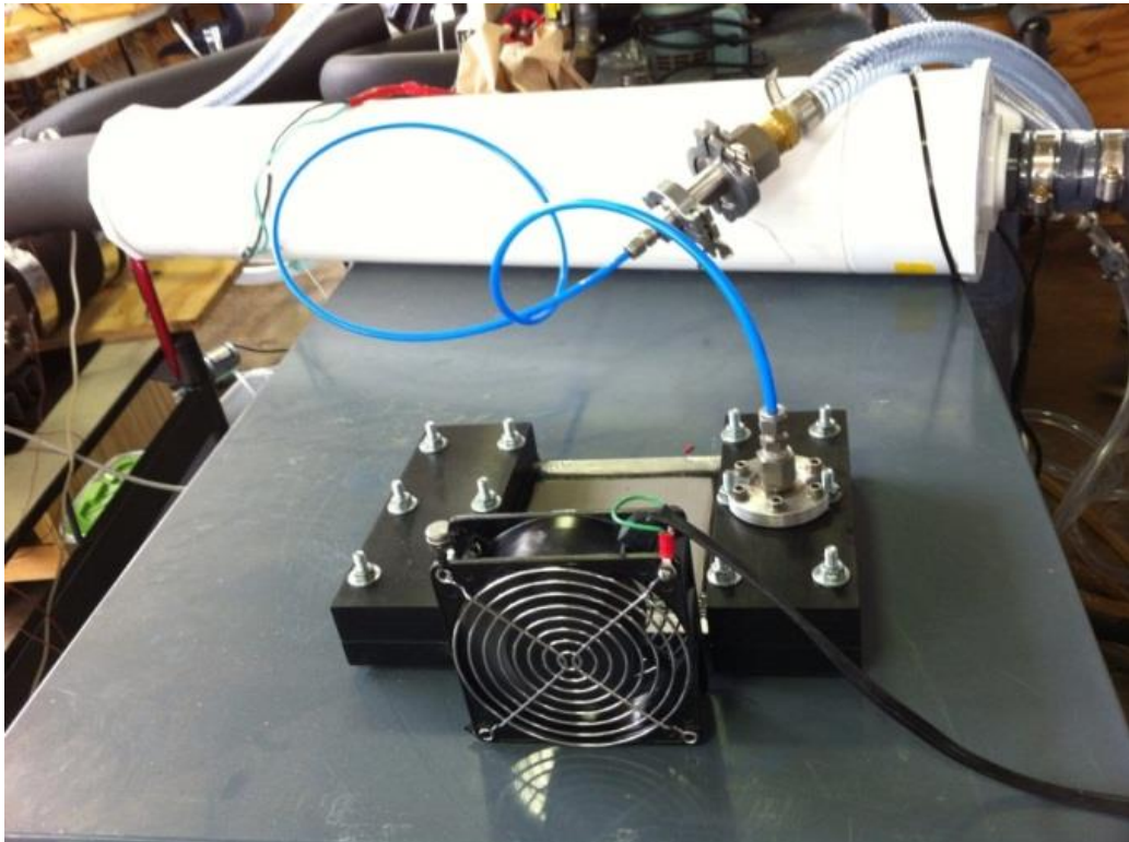
Figure 95. Membrane Cassette #3 test with 1/4-inch pipe connection
