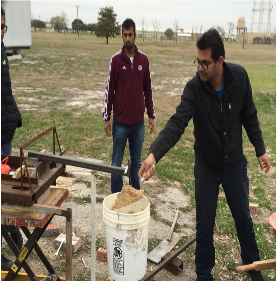
Figure 26: A bucket used to apply sand load to end of bond wrench moment arm
