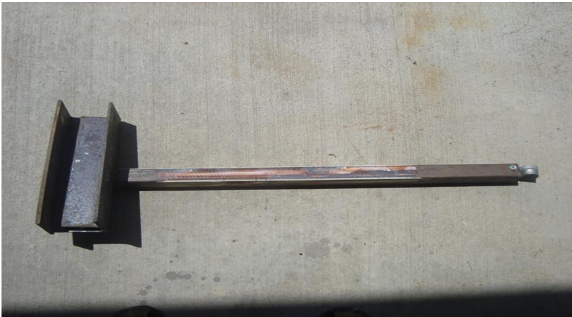
Figure 13: TAMU Unbalanced Bond Wrench by Chaudhari (2010)
