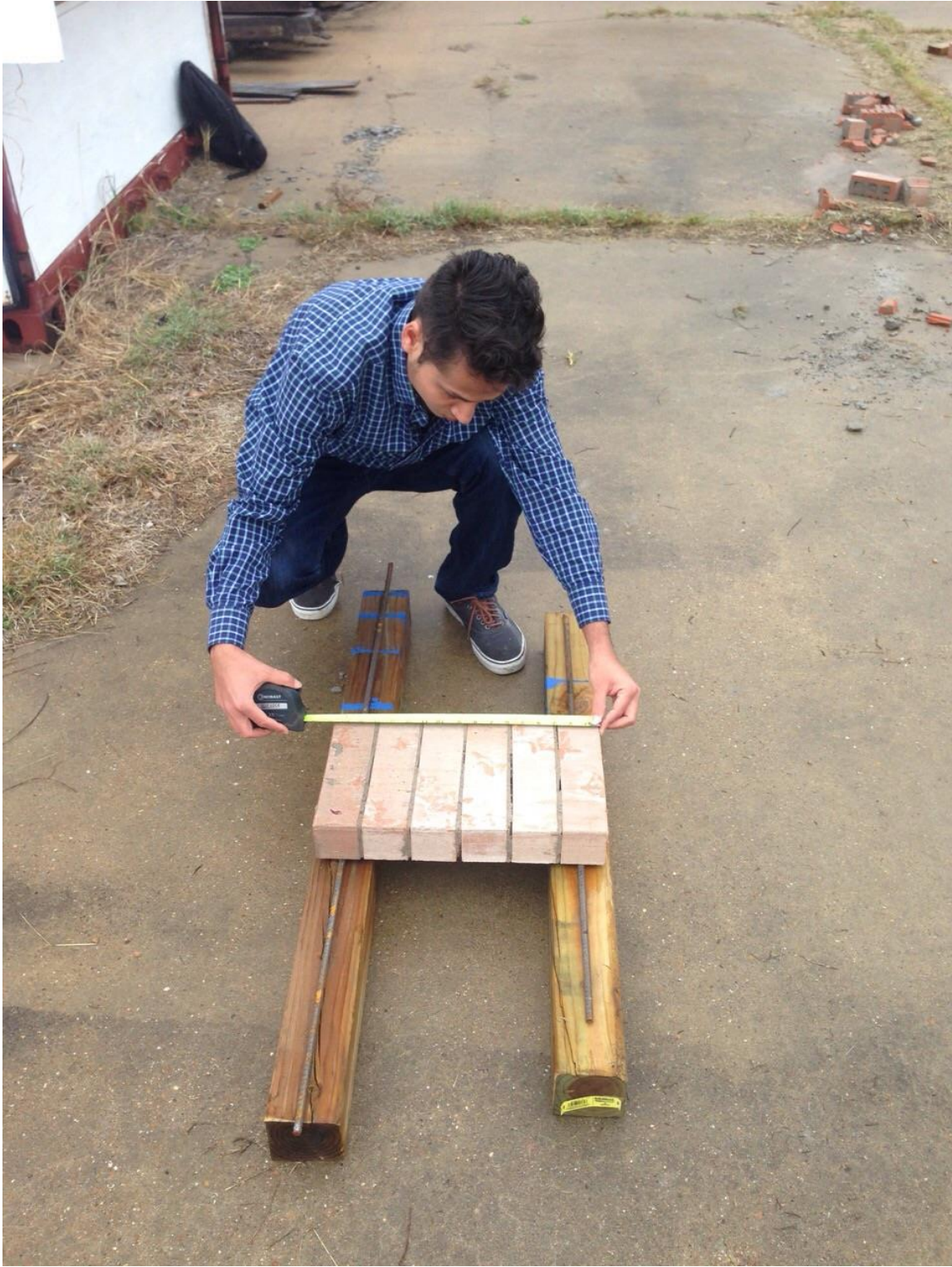
Figure 29: Equivalent ASTM E518 arrangement
