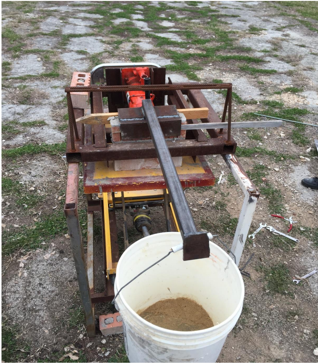
Figure 25: Setup of the frame and hydraulic table for placing bricks to be tested
