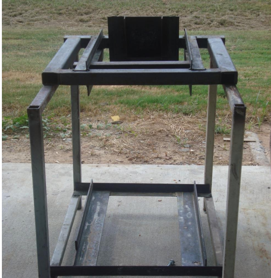
Figure 23: Steel frame for the bond wrench experiment
