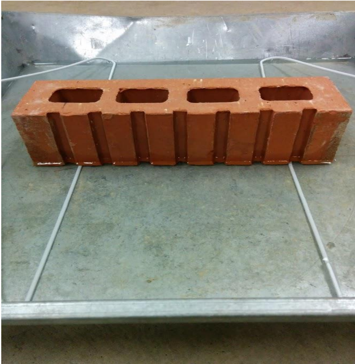
Figure 31: Absorption test on sample brick
