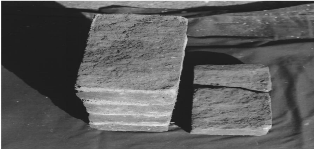
Figure 15: Bond failure when the mortar is still intact (Sarangapani et al., 2005)
