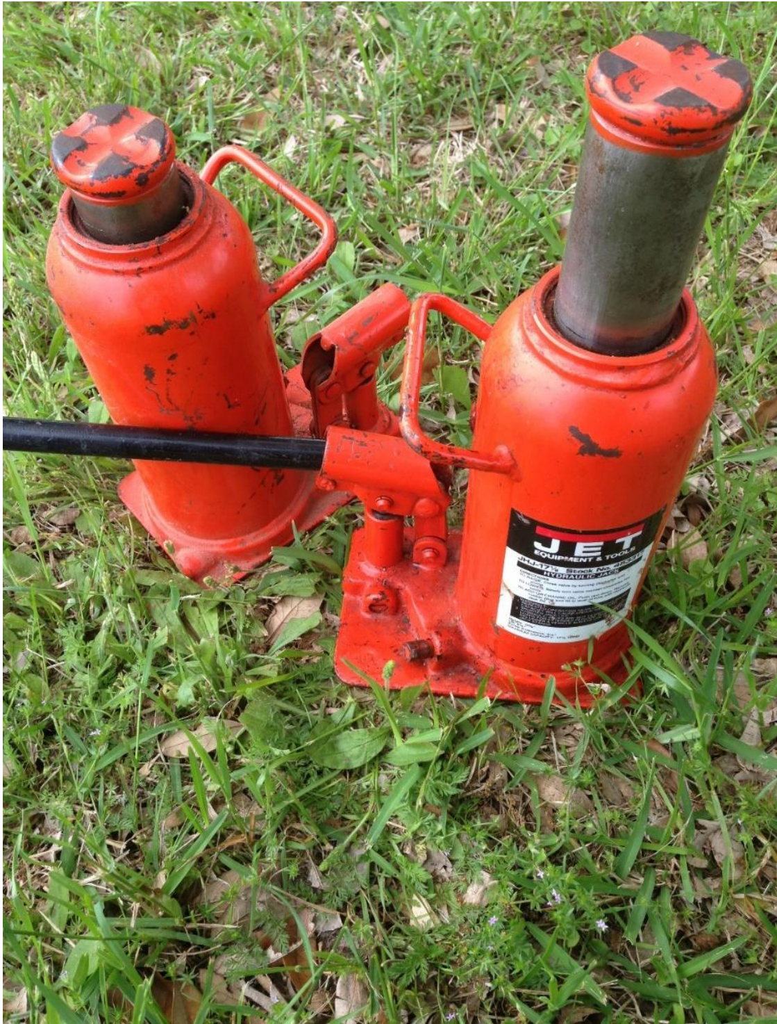
Figure 24: Hydraulic Jack to lift the specimen
