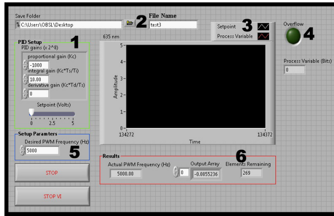
Figure G7: A screen capture of the front panel schematic for the host PC PID control VI.
