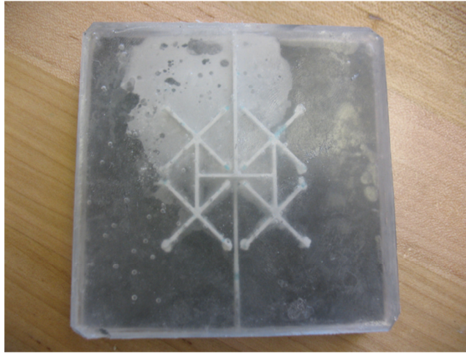
Figure 8 The internal pressure created by the fluids caused the channel bonding to fail [45].
