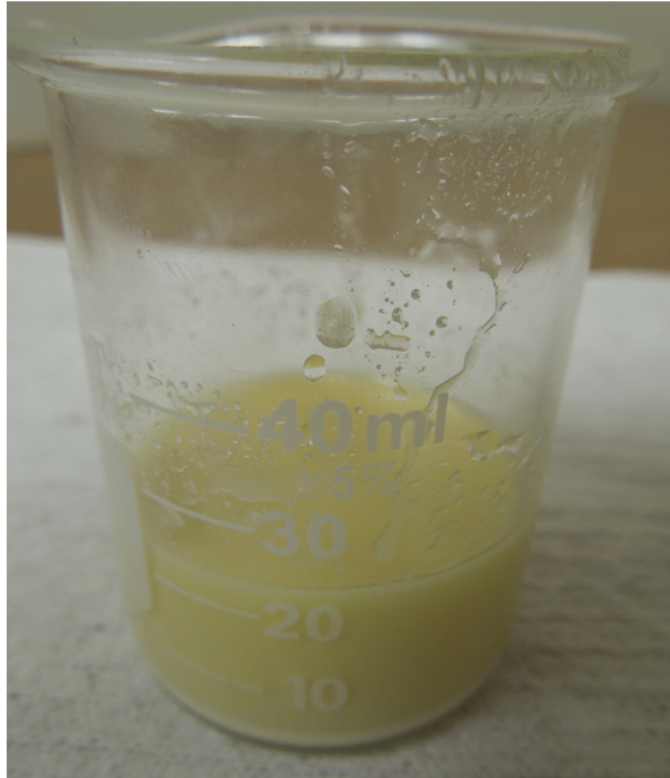
Figure 80 Hydrocal 2400 doped with BSTO particles after 50 minutes. The white ring at the bottom of the beaker is from BSTO particles that have settled.
