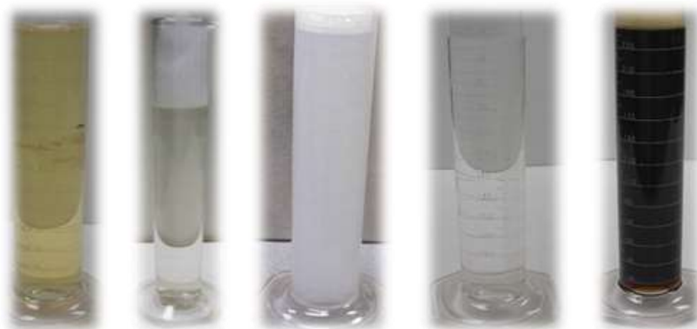
Fig. 19—Compatibility of dispersants solutions (1.6 wt%). From left to right are dispersants A01, A05, A10, B13, and C26.
