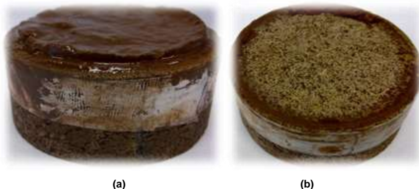
Fig. 51—Single-step procedure to dissolve Mn_3O_4 -based filter cake at 250°F. Pictures showed filter cake (a) before reaction, (b) after HCl/glycolic acid reaction. The HCl and glycolic acids concentrations were 1 and 7 wt%.
