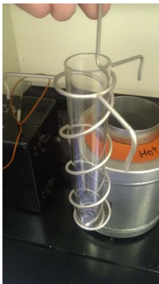
Figure 9: Image of the 22 mm x 300 mm glass tube in the steel cradle.
