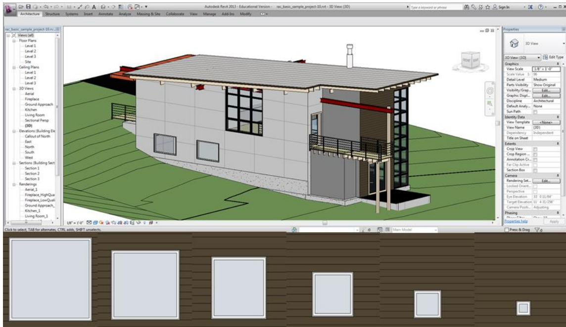
Figure 9. The BIM model of the case study with different window sizes that can be parametrically changed by PBES
