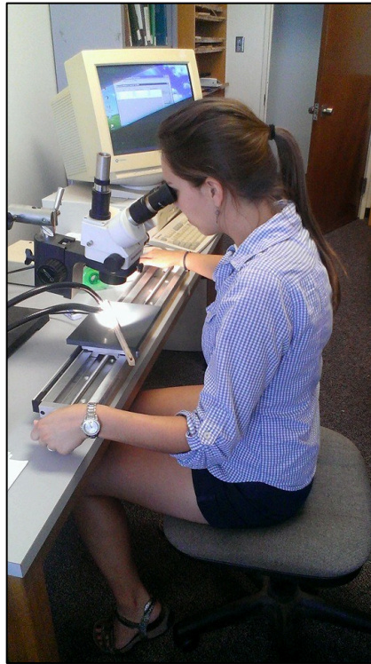
Figure 26. Measuring a tree ring series using a stereomicroscope and Velmex system.
