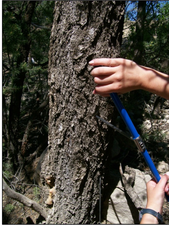
Figure 23. Using an increment borer to core a tree at breast height.
