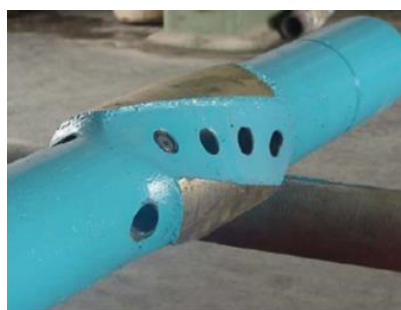
Fig. 16 Acid Jetting Assembly (Sasongko et al. 2011)
