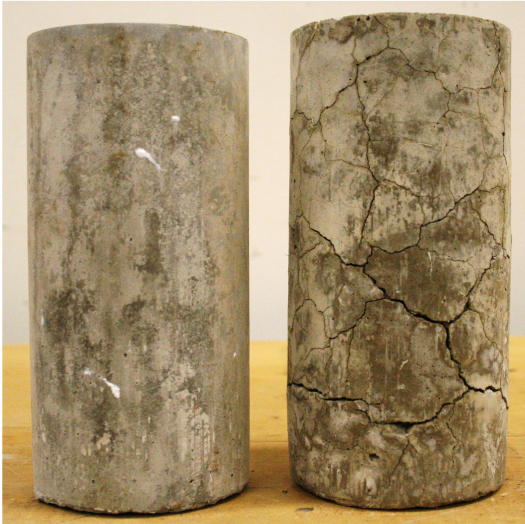
(a) Wet-Room Cured Cylinder
