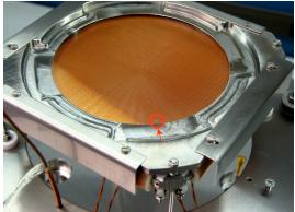
(b) The delay line anode
