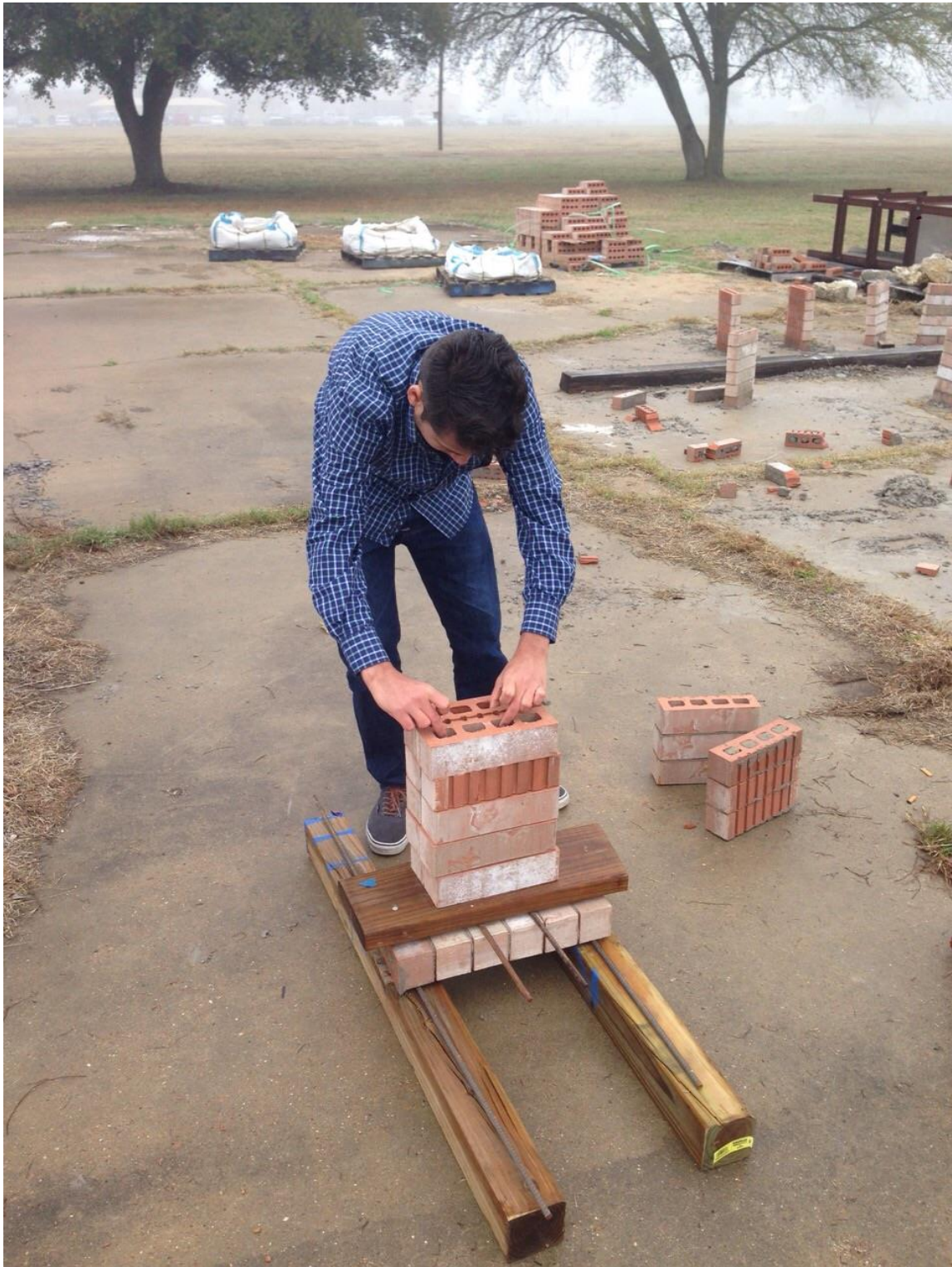
Figure 30: Loading the specimen
