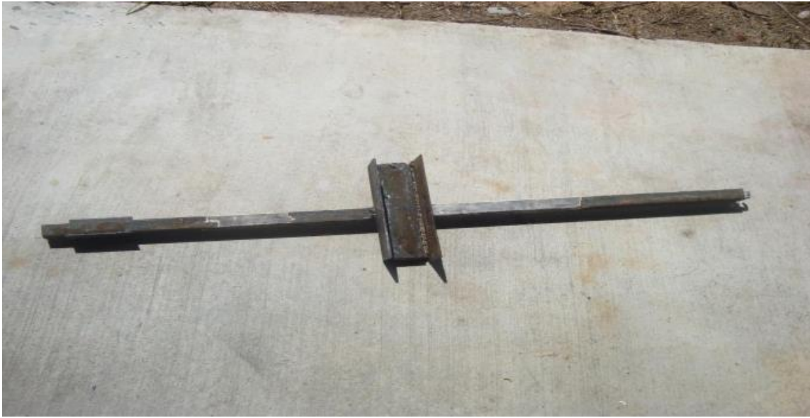
Figure 12: TAMU balanced bond wrench by Chaudhari (2010)
