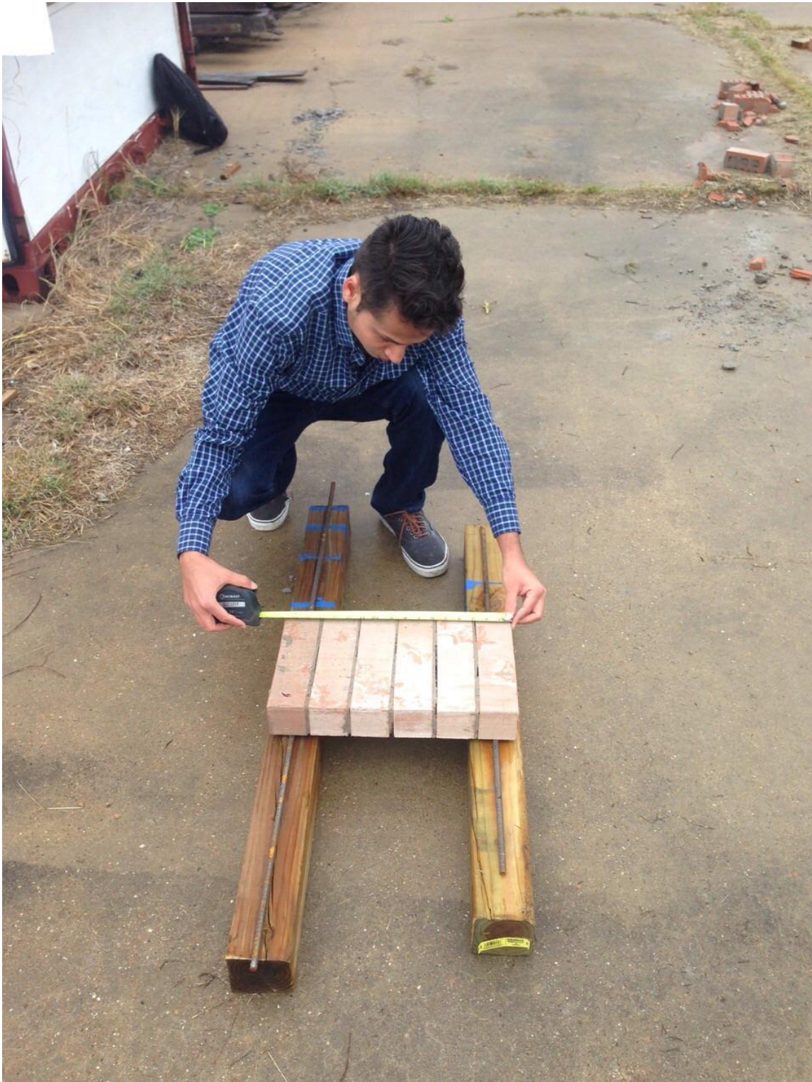
Figure 29: Equivalent ASTM E518 arrangement
