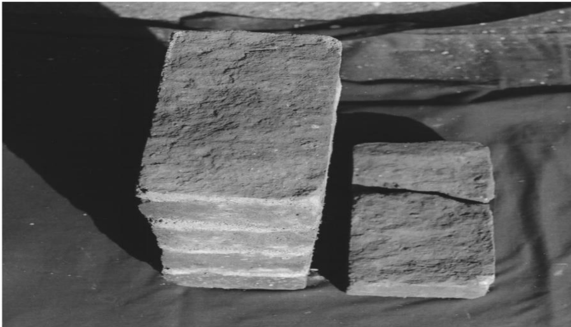
Figure 15: Bond failure when the mortar is still intact (Sarangapani et al., 2005)
