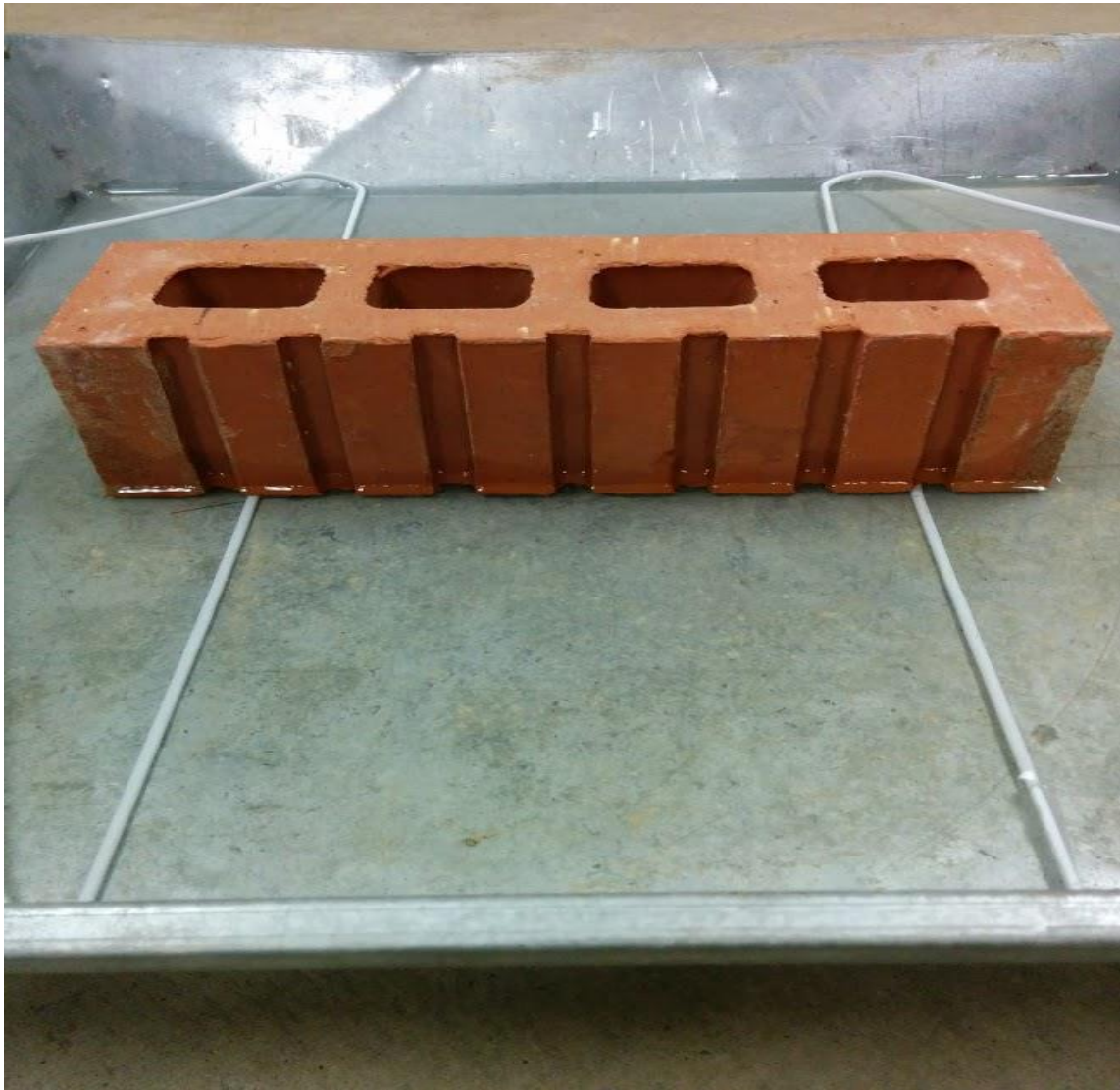
Figure 31: Absorption test on sample brick
