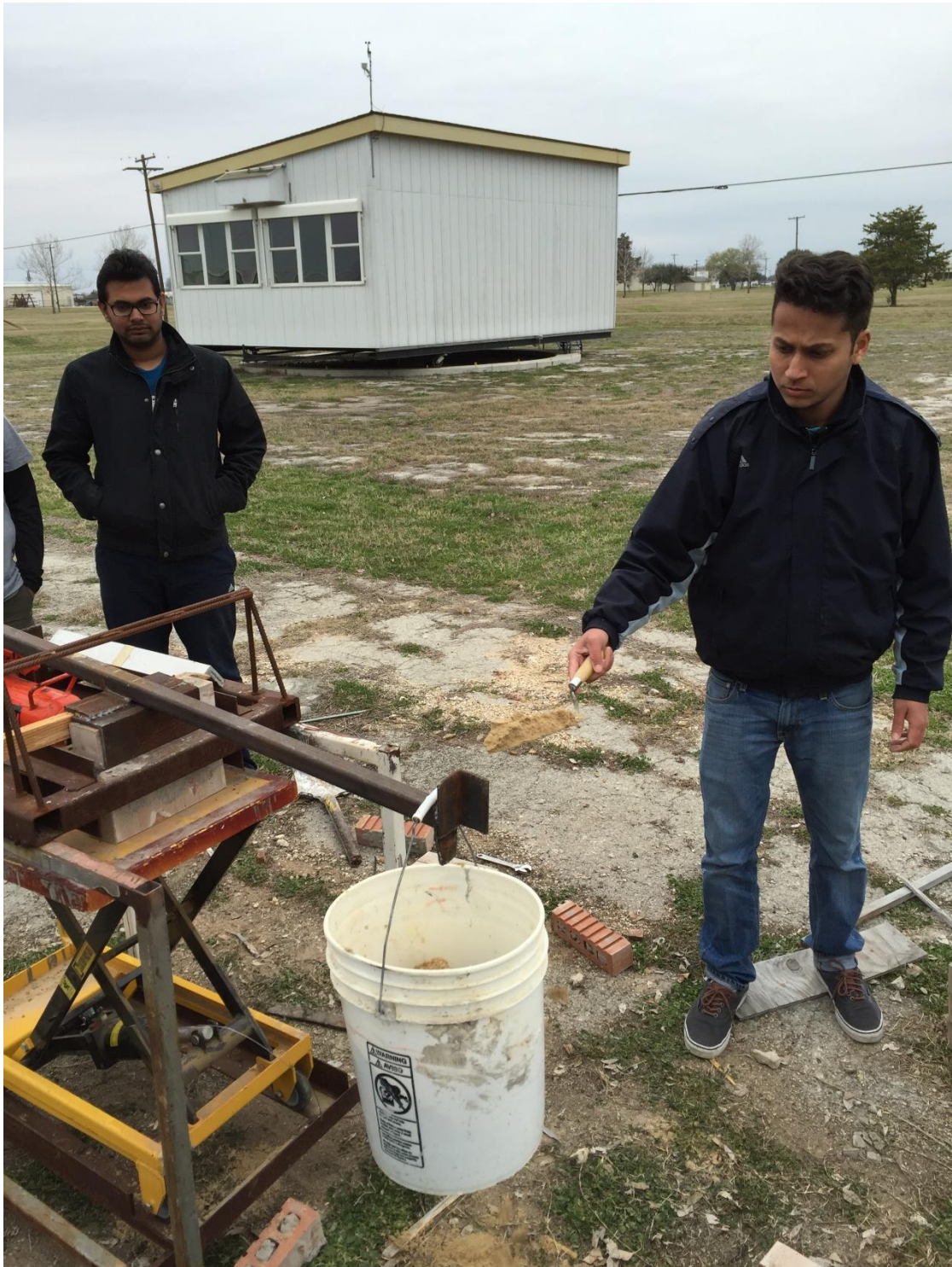
Figure 26: A bucket used to apply sand load to end of bond wrench moment arm
