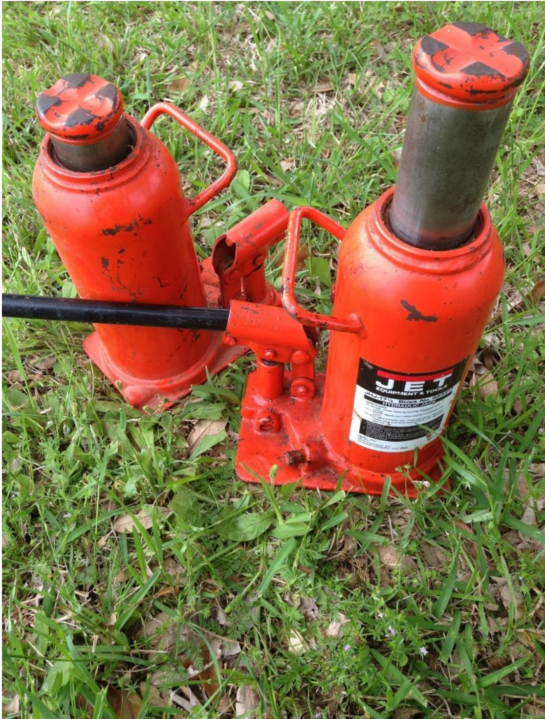
Figure 24: Hydraulic Jack to lift the specimen
