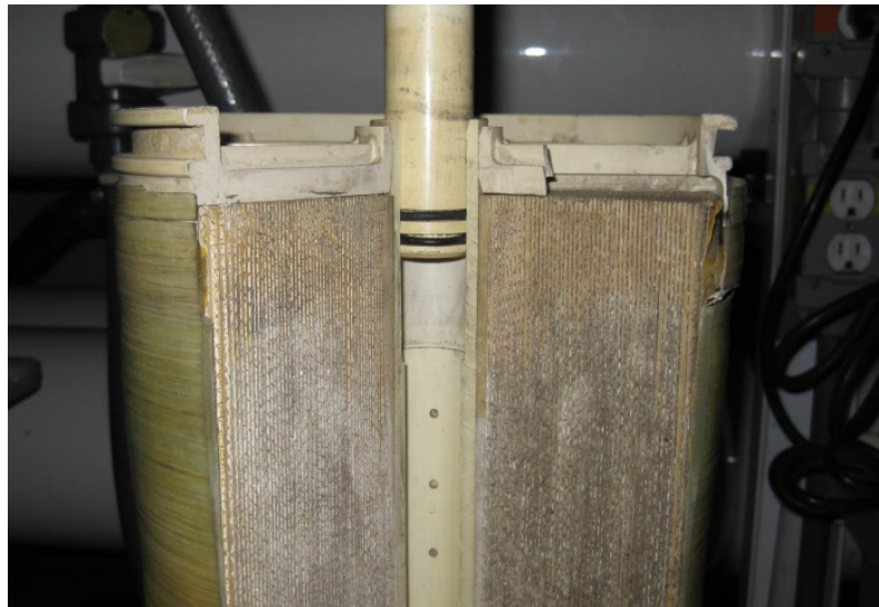
Figure A- 71: Section cut-out of an RO filter showing its many layers.
