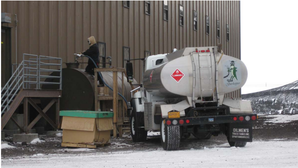
Figure 25: A McMurdo fuelie refills the fuel tank alongside one of the uppercase dorms. The type of truck is a “gasshopper.” Photo by author, 2009.
