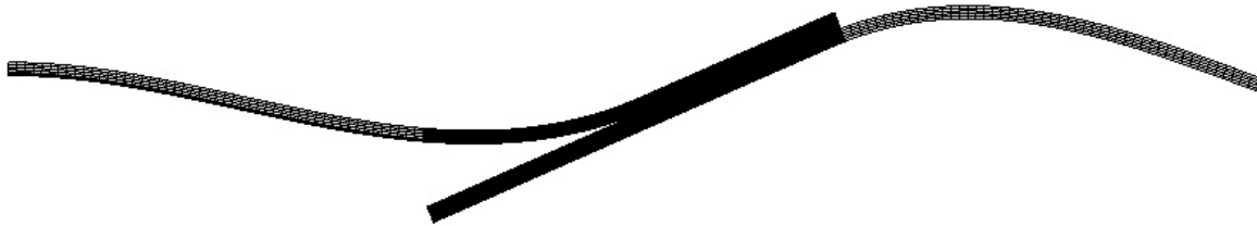
Fig. 28 Deformed shape of a single lap joint with and interface crack.
