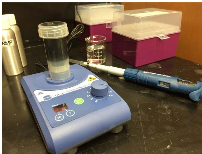
Figure 9. Electrode slurry mixing on IKA mixer. A two-stage mix is utilized, where the solvent is mixed with the dry powder, and is again mixed after adding the 10% by weight binder solution.
