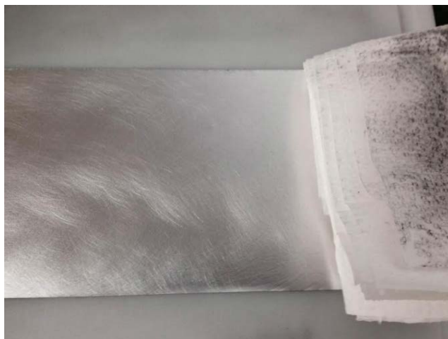
Figure 10. Cleaned aluminum substrate with residue shown on paper towel.
