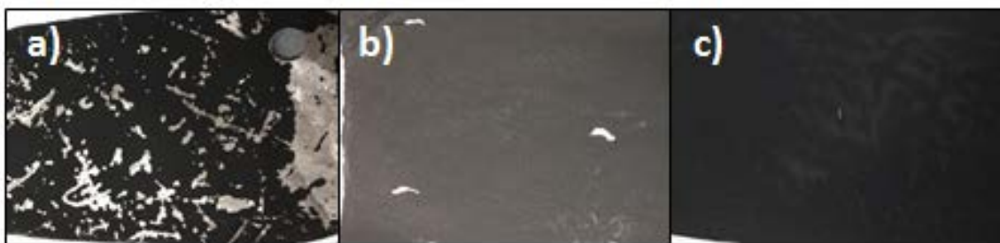
Figure 12. Electrode sheets: a) with too little NMP, b) with too much NMP, and c) with non-uniform drying.
