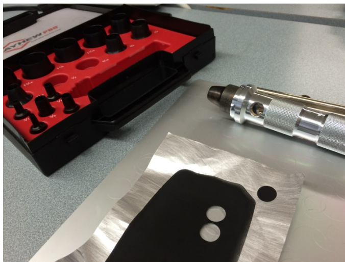
Figure 13. Electrode sheet shown with punched out cathode.
