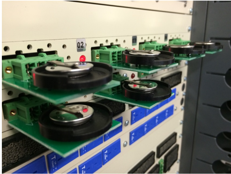
Figure 16. Coin cells undergoing cycling (charge/discharge at different rates) on the Arbin system.
