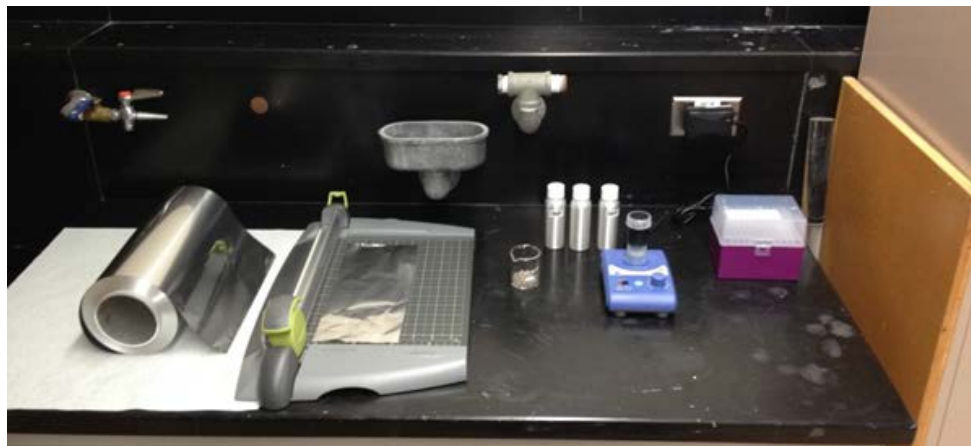
Figure 3. Electrode substrate and slurry preparation station.
