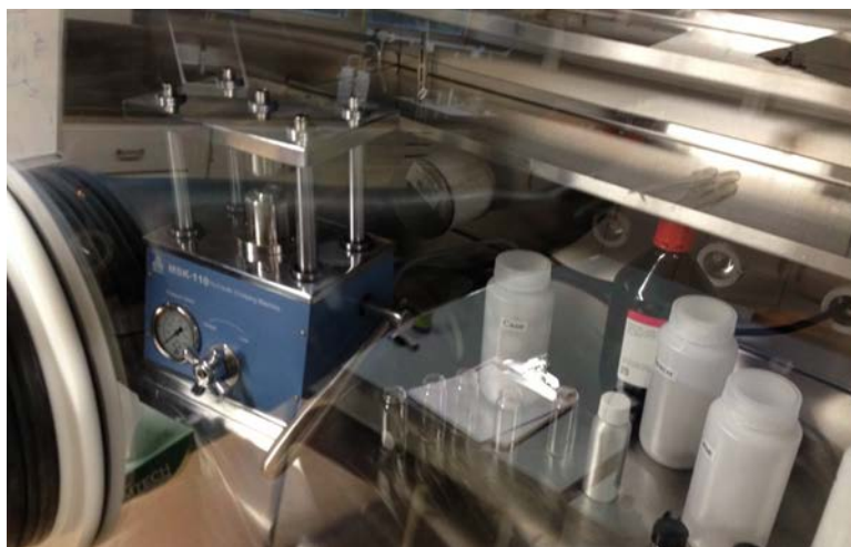
Figure 6. Coin cell crimper pictured within glovebox.
