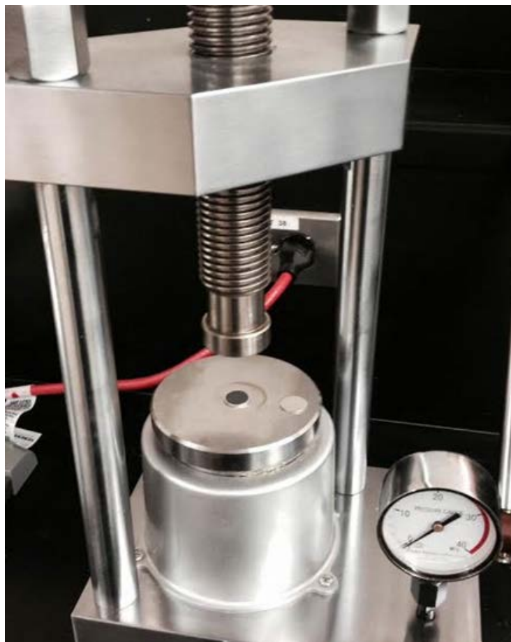
Figure 27. Lab press shown with electrode sample on stainless steel spacer.
