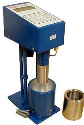
Fig. 8—M3600 grace viscometer (Grace Instrument Industries LLC 2014).
