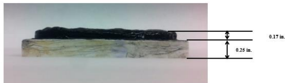
Fig. 23—Filter cake of KNO 3 -based drilling fluid using ilmenite as the weighting material (Formula 12).
