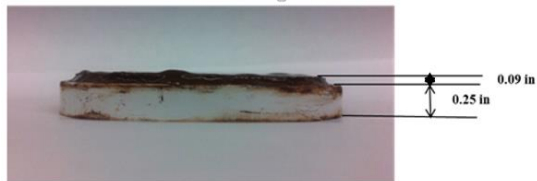
Fig. 20—Filter cake of \text{KNO}_3 -based drilling fluid using \text{Mn}_3\text{O}_4 as the weighting material (Formula 9).
