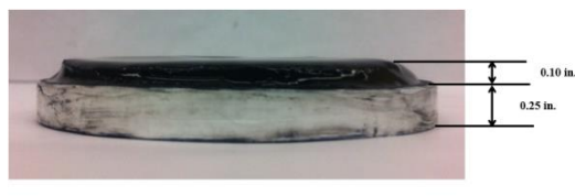
Fig. 22—Filter cake of KNO 3 -based drilling fluid using ilmenite as the weighting material (Formula 11).
