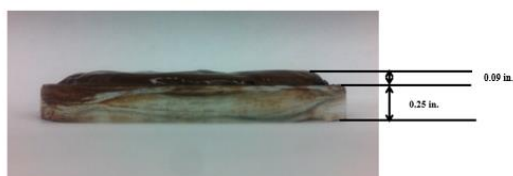
Fig. 15—Filter cake of KCl-based drilling fluid using Mn_3O_4 as the weighting material (Formula 4).
