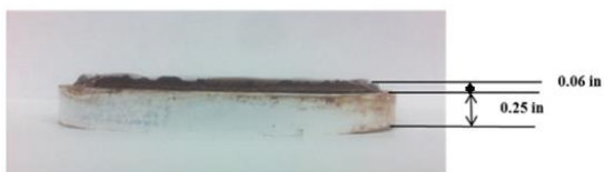
Fig. 14—Filter cake of KCl-based drilling fluid using Mn_3O_4 as the weighting material (Formula 3).
