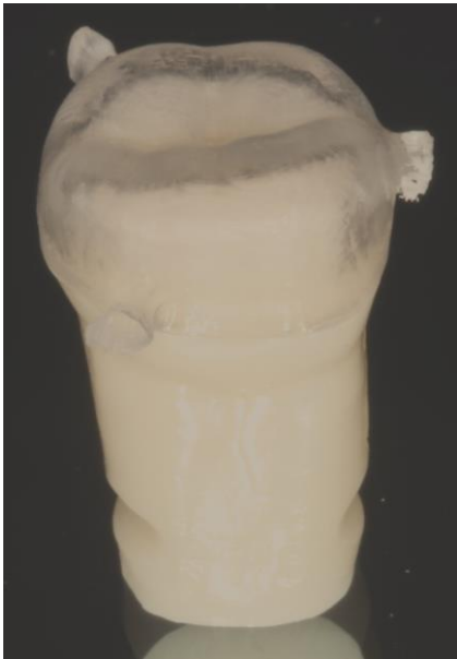
Figure 2: Polycon® cast coping seated onto master epoxy resin die prior to pressing.
