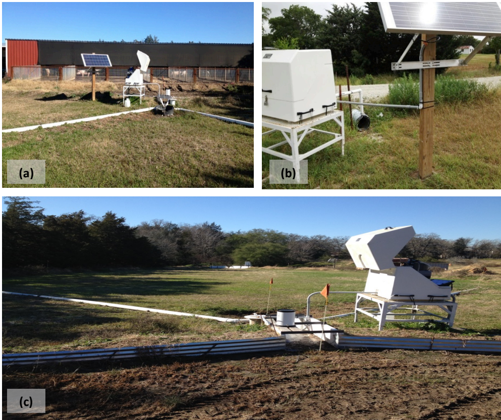
Figure 3. Brazos County site (a) view of pens above flume at “VTA In,” (b) culvert through which “Control” site drains, and (c) entire VTA with runoff distribution system.
